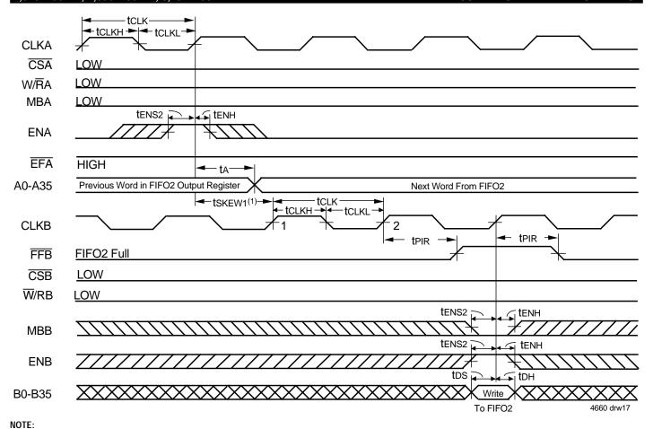
1. tskew1 is the minimum time between a rising CLKA edge and a rising CLKB edge for FFB to transition HIGH in the next CLKB cycle. If the time between the rising CLKA edge and rising CLKB edge is less than tskew1, then FFB may transition HIGH one CLKB cycle later than shown.
