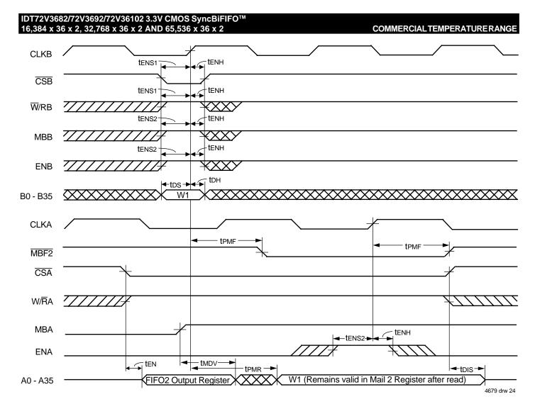
Figure 21. Timing for Mail2 Register and MBF2 Flag (IDT Standard and FWFT Modes)
