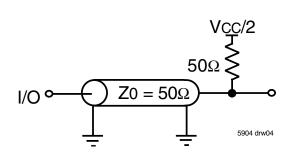
Figure 2a. AC Test Load
