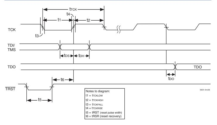
Figure 35. Standard JTAG Timing
