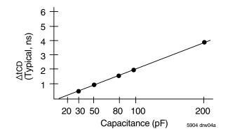
Figure 2b. Lumped Capacitive Load, Typical Derating
