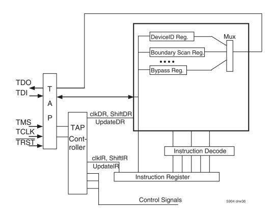
Figure 33. Boundary Scan Architecture
