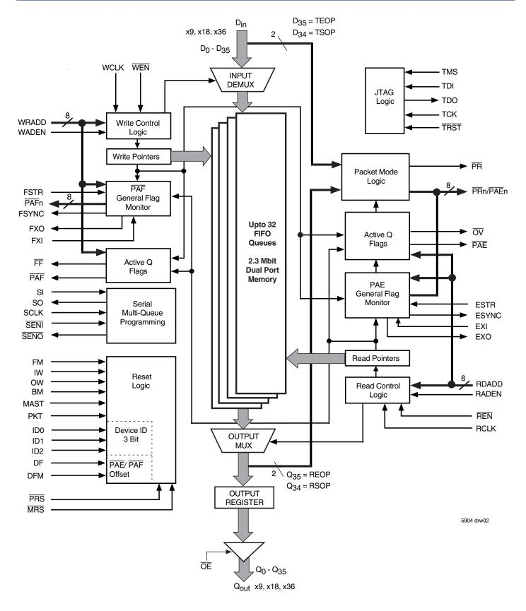
Figure 1. Multi-Queue Flow-Control Device Block Diagram
