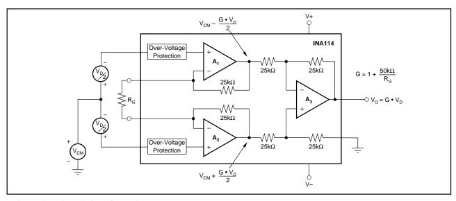
FIGURE 4. Voltage Swing of A<sub>1</sub> and A<sub>2</sub>.
