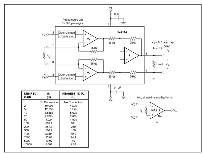
FIGURE 1. Basic Connections.
