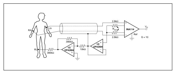
FIGURE 10. ECG Amplifier With Right-Leg Drive.
