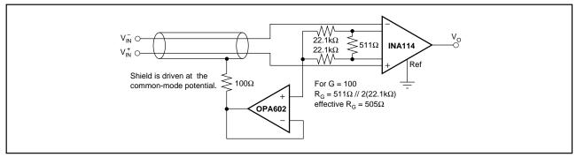
FIGURE 7. Shield Driver Circuit.
