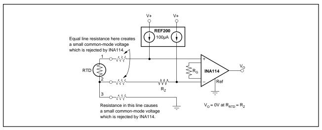
FIGURE 8. RTD Temperature Measurement Circuit.
