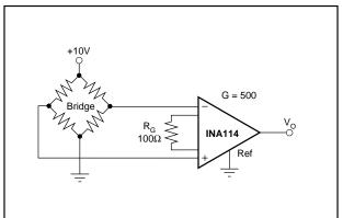
FIGURE 11. Bridge Transducer Amplifier.
