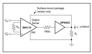
FIGURE 6. Buffered Output for Heavy Loads.
