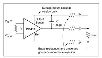
FIGURE 5. Remote Load and Ground Sensing.
