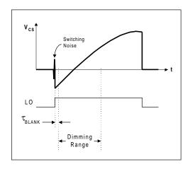
Figure 15, Current sense timing diagram.
