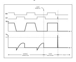
Figure 18, hard-switching with latch off
