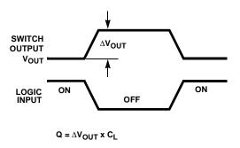
FIGURE 1. SWITCHING TIMES
