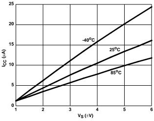
FIGURE 17. SUPPLY CURRENT vs SUPPLY VOLTAGE
