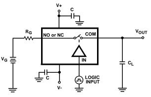
FIGURE 2A. MEASUREMENT POINTS
