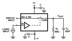
$C_{\mbox{L}}$  includes fixture and stray capacitance.
