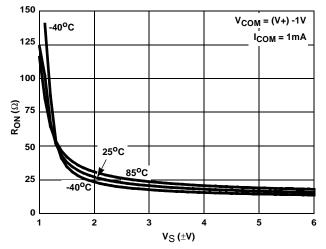
FIGURE 7. ON RESISTANCE vs SUPPLY VOLTAGE
