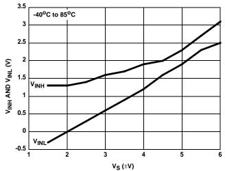
FIGURE 13. DIGITAL SWITCHING POINT vs SUPPLY VOLTAGE
