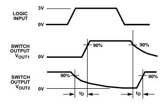
FIGURE 3A. MEASUREMENT POINTS
