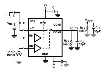
$\mathsf{C}_{\mathsf{L}}$  includes fixture and stray capacitance. Reconfigure accordingly to test SW3 and SW4.
