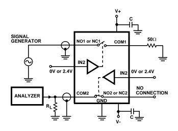
FIGURE 6. CROSSTALK TEST CIRCUIT
