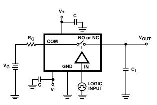
Repeat test for all switches.  $\ensuremath{\mathsf{C}}_L$  includes fixture and stray capacitance.
