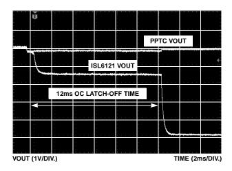
FIGURE 15. ISL6121 vs PPTC INTO 1.6 $\Omega$  LOAD
