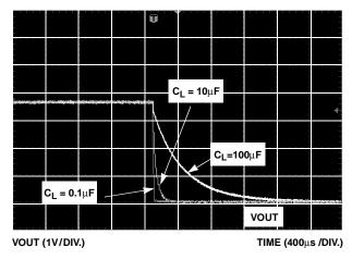
FIGURE 10. FAST TURN-OFF vs CLOAD
