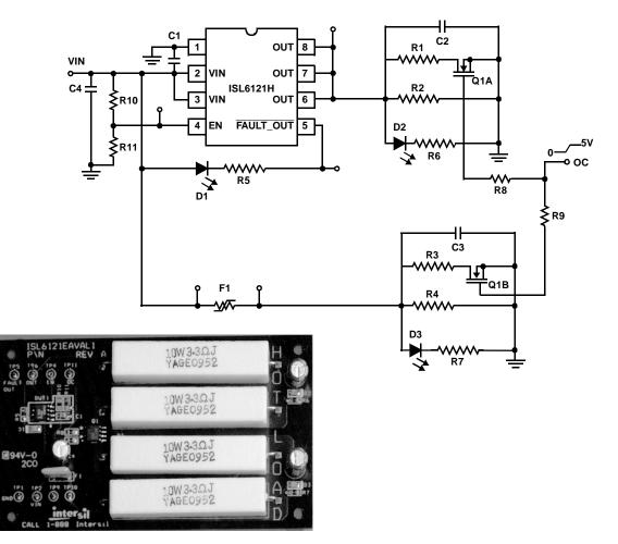
FIGURE 17. ISL6121EVAL1 SCHEMATIC AND PHOTOGRAPH
