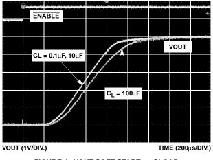
FIGURE 4. VOUT SOFT START vs CLOAD
