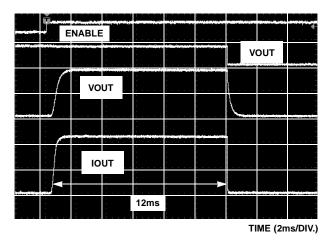
FIGURE 11. ISL6121 TURN-ON INTO 3A OC
