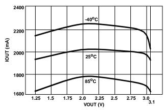
FIGURE 5. CURRENT REGULATION vs VOUT (VIN = 3.3V)
