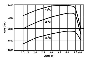
FIGURE 6. CURRENT REGULATION vs VOUT (VIN = 5.0V)
