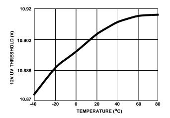
FIGURE 6. 12V UV THRESHOLD
