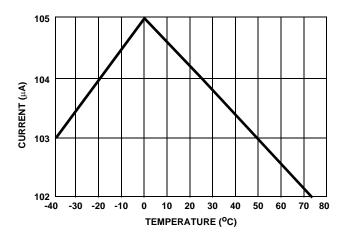
FIGURE 3.  $R_{ILIM}$  SOURCE CURRENT
