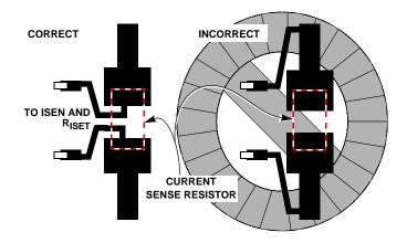
FIGURE 1. SENSE RESISTOR PCB LAYOUT
