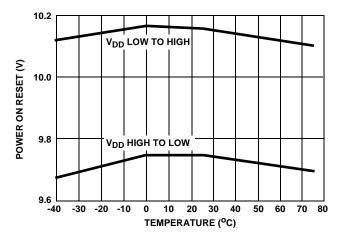
FIGURE 12. POWER ON RESET VOLTAGE THRESHOLD
