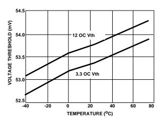
FIGURE 10. OC VOLTAGE THRESHOLD WITH RLIM =  $5k\Omega$
