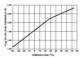
FIGURE 5.  $C_{TIM}$  OC VOLTAGE THRESHOLD
