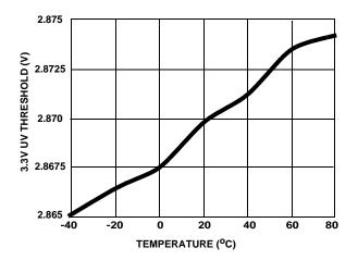
FIGURE 7. 3.3V UV THRESHOLD
