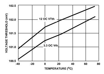
FIGURE 11. OC VOLTAGE THRESHOLD WITH  $R_{\mbox{\scriptsize LIM}}$  = 10k $\!\Omega$
