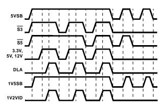
FIGURE 6. 1.5V<sub>SB</sub>, AND 1.2V<sub>VID</sub> TIMING DIAGRAM
