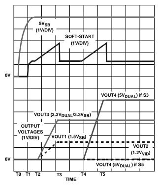
FIGURE 7. SOFT-START INTERVAL IN A SLEEP STATE; ISL6504
