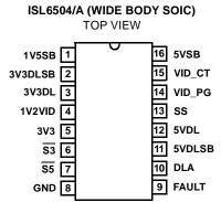
NOTE: SOIC Layout should accomodate both wide and narrow footprints
