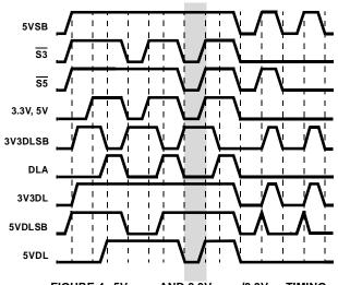
FIGURE 4. 5V<sub>DUAL</sub> AND 3.3V<sub>DUAL</sub>/3.3V<sub>SB</sub> TIMING DIAGRAM; ISL6504
