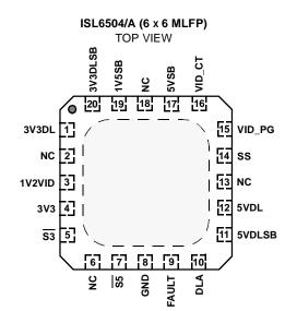
NOTE: The MLFP bottom pad is electrically connected to the IC substrate, at GND potential. It can be left unconnected, or connected to GND; do NOT connect to another potential.
