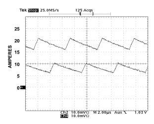
FIGURE 8. TWO CHANNEL multi-phase SYSTEM WITH CURRENT BALANCING DISABLED
