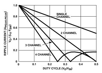
FIGURE 12. RIPPLE CURRENT vs DUTY CYCLE
