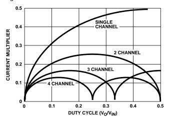
FIGURE 13. CURRENT MULTIPLIER vs DUTY CYCLE
