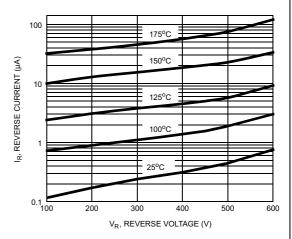
Figure 2. Reverse Current vs Reverse Voltage
