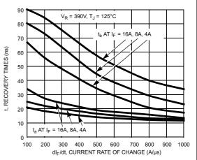
Figure 4.  $t_a$  and  $t_b$  Curves vs  $dI_F/dt$
