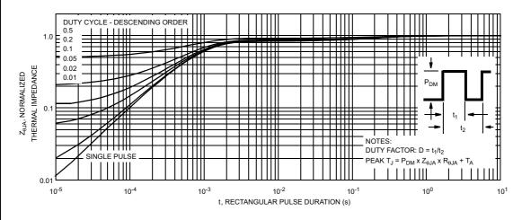
Figure 11. Normalized Maximum Transient Thermal Impedance
