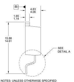
A) ALL DIMENSIONS ARE IN MILLIMETERS. B) REFERENCE JEDEC, TO-263, VARIATION AB.
