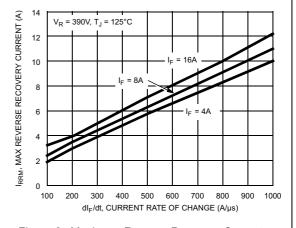
Figure 6. Maximum Reverse Recovery Current vs  $\mathrm{dI}_{\mathrm{F}}/\mathrm{dt}$
