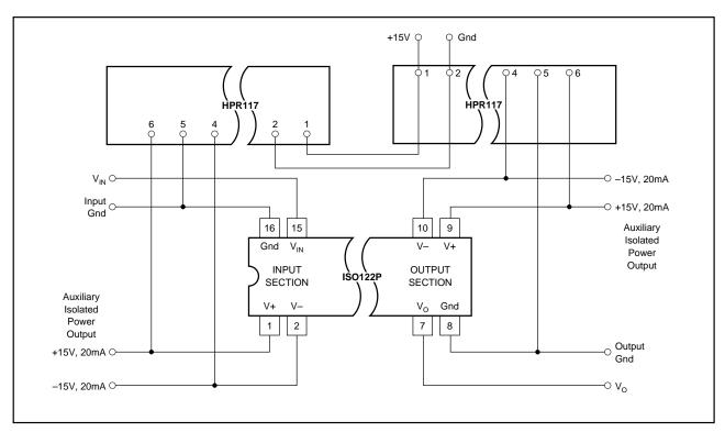
FIGURE 13. Powered ISO Amp with Three-Port Isolation. For additional information refer to AB-024.
