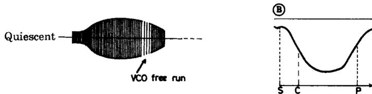
Note : Error will occur in the measurement of the selectivity characteristics if the video frequency changes between (A) and (C) (by a video equalizer, etc.)
