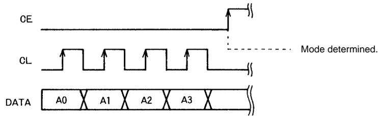
1. In the serial data input modes (modes 1 and 2),  $t_1 \geq 1.5 \mu\text{s}$ ,  $t_2 \geq 0 \mu\text{s}$ ,  $t_3 \geq 1.5 \mu\text{s}$ , and  $t_4 < 1.5 \mu\text{s}$ .
