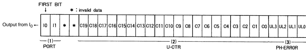
The LC7216M includes a 28-bit internal shift register that can be used to output the following data from DO: the IN0 and IN1 input port states, the general-purpose counter (20-bit binary counter) and the unlock detection circuit state. The contents of the shift register is latched at the point that serial data output mode is selected.
