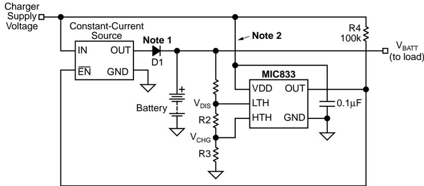
**Note 1.** D1 may not be required. It is shown here to indicate the disabled current source should not load the battery.
