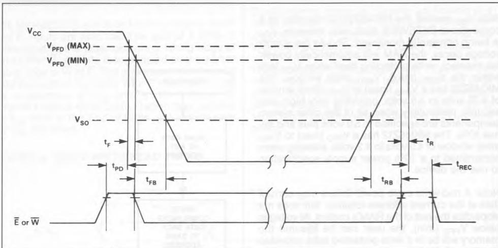
**DC ELECTRICAL CHARACTERISTICS (POWER-DOWN/POWER-UP TRIP POINT VOLTAGES)**
