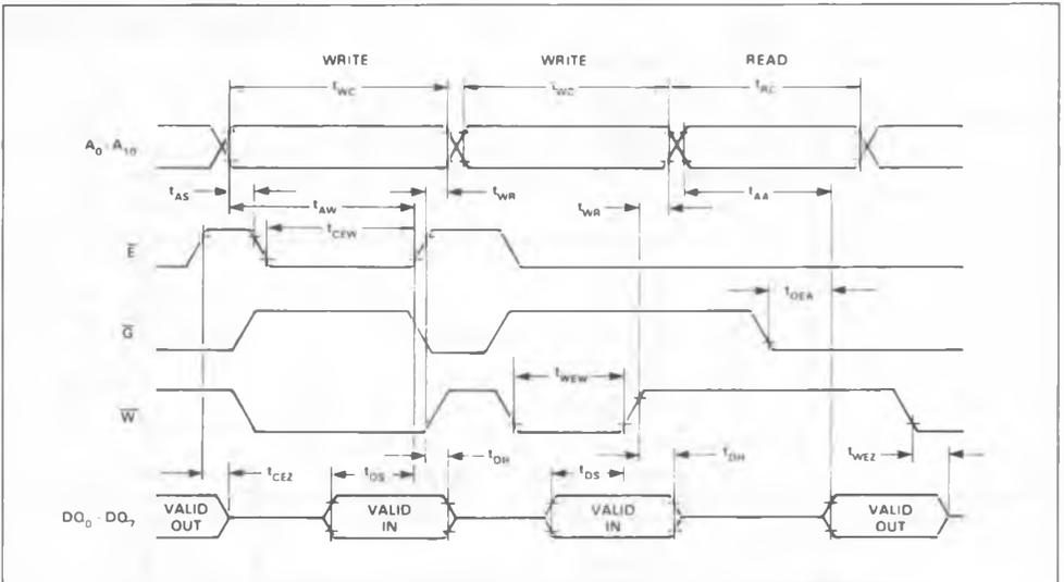
**AC ELECTRICAL CHARACTERISTICS (WRITE CYCLE TIMING)**
