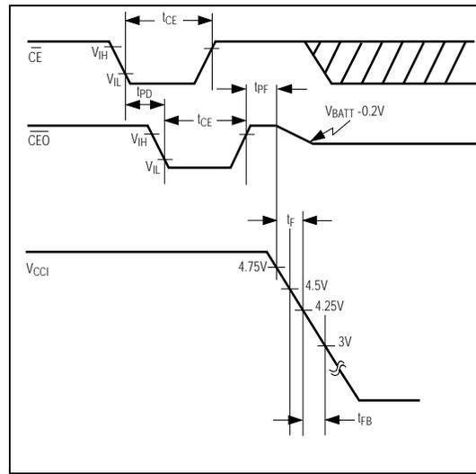
Figure 3. Power-Down Timing Diagram
