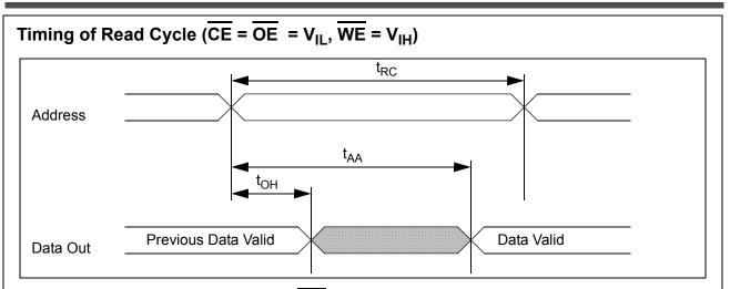
Timing Waveform of Read Cycle ( $\overline{WE} = V_{IH}$ )
