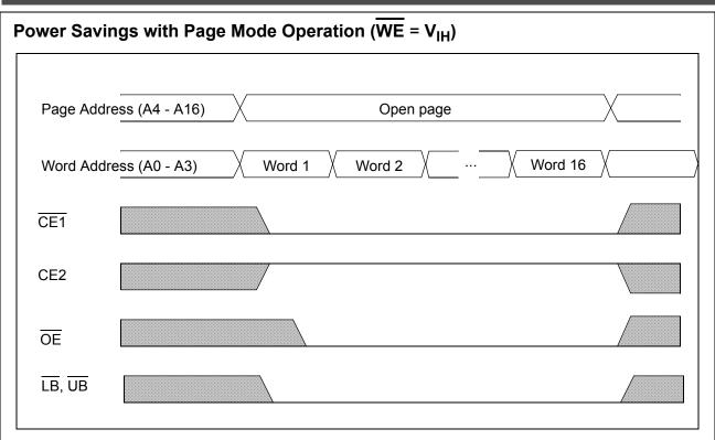
Note: Page mode operation is a method of addressing the SRAM to save operating current. The internal organization of the SRAM is optimized to allow this unique operating mode to be used as a valuable power saving feature.
