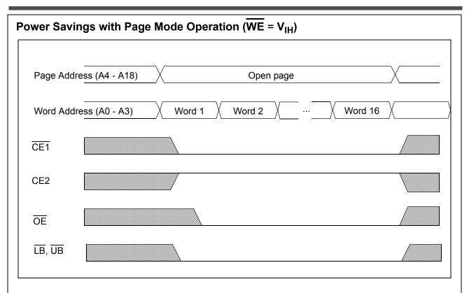
Note: Page mode operation is a method of addressing the SRAM to save operating current. The internal organization of the SRAM is optimized to allow this unique operating mode to be used as a valuable power saving feature.
