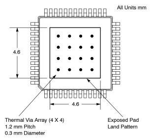
Figure 7. Recommended Thermal Land Pattern
