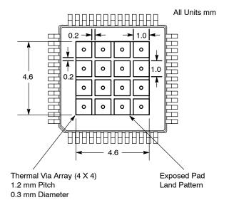
Figure 8. Recommended Solder Mask Openings
