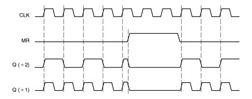
Figure 4. Master Reset (MR) Timing Diagram
