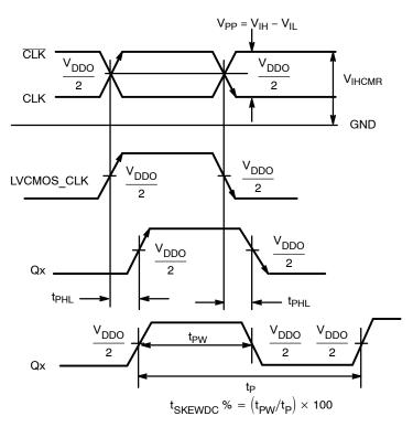
Figure 4. AC Reference Measurement
