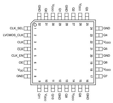
Figure 2. Pinout Configuration (Top View)
