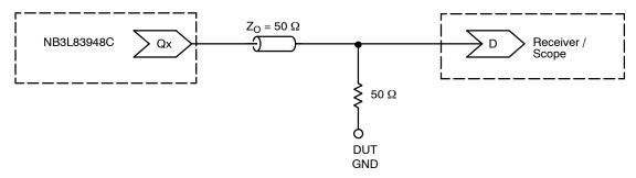
Figure 5. Typical Termination for Output Driver and Device Evaluation. Supplies may be centered on GND  $(\pm\,1.65$  V or  $\pm\,1.25$  V) to permit direct connection into 50  $\Omega$  to GND Scope modules
