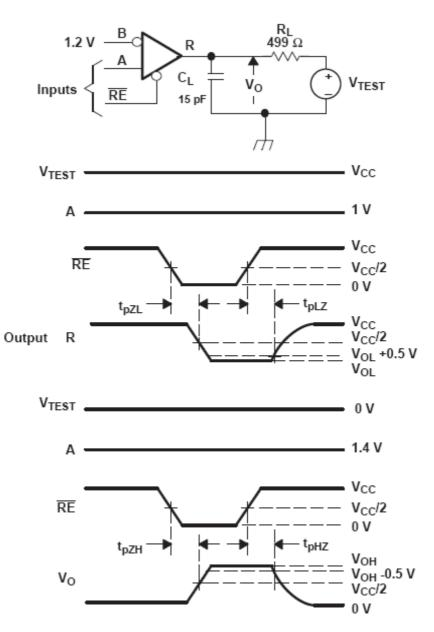
A. All input pulses are supplied by a generator having the following characteristics: tr or tr $\leq$  1 ns, frequency = 500 kHz, duty cycle = 50 ±5%.
