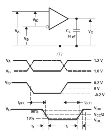
A. All input pulses are supplied by a generator having the following characteristics: tr or tr  $\leq$  1 ns, frequency = 50 MHz, duty cycle = 50  $\pm$ 5%. CL is a combination of a 20%-tolerance, low-loss ceramic, surface-mount capacitor and fixture capacitance within 2 cm of the D.U.T.
