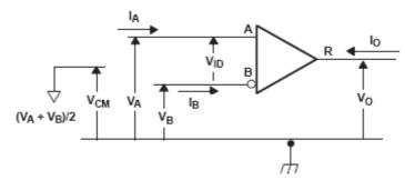
Figure 11. Receiver Voltage and Current Definitions
