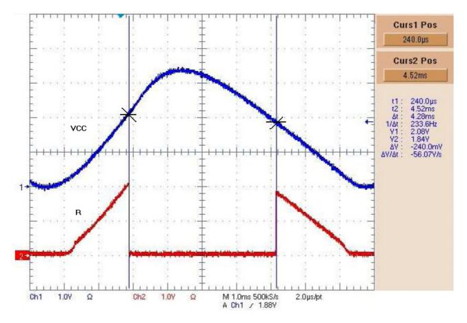
Figure 17. M-LVDS Receiver Output: VCC (CHANNEL 1), R Pin (CHANNEL 2)
