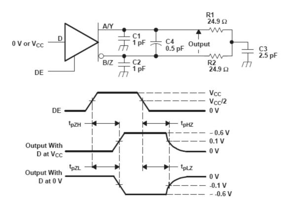
A. All input pulses are supplied by a generator having the following characteristics: tr or tr≤ 1 ns, frequency = 500 kHz, duty cycle =  $50 \pm 5\%$ .
