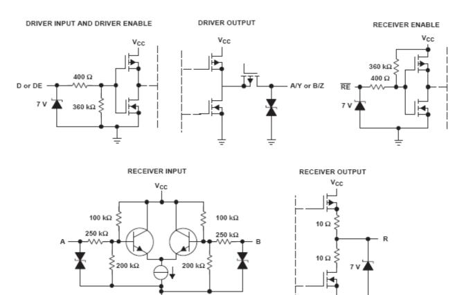
Figure 15. Equivalent Input and Output Schematic Diagrams
