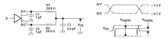
A. All input pulses are supplied by a generator having the following characteristics: tr or tr $\leq$  1 ns, pulse frequency = 500 kHz, duty cycle = 50 ± 5%.
