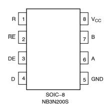
Figure 2. Pinout Diagrams (Top View)
