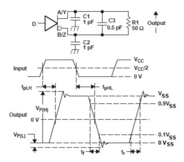
A. All input pulses are supplied by a generator having the following characteristics: tr or tr $\leq$  1 ns, frequency = 500 kHz, duty cycle = 50 ±5%.
