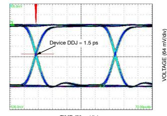
TIME (72 ps/div) Figure 9. Typical Output Waveform at 2.488 Gb/s with PRBS  $2^{23}$ –1 (V<sub>INPP</sub> = 400 mV; Input Signal DDJ = 12 ps)
