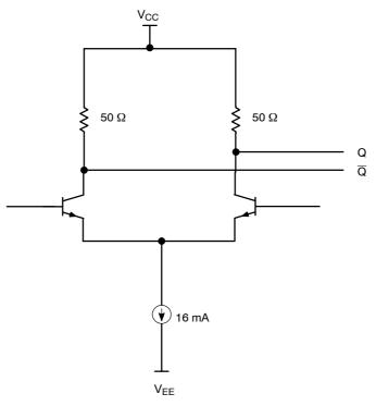
Figure 19. CML Output Structure
