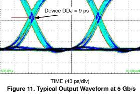
with PRBS 223–1 (VINPP = 400 mV; Input Signal DDJ = 13 ps)
