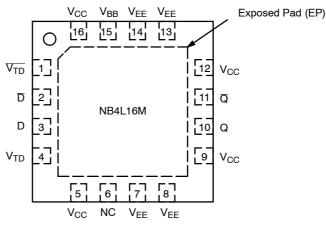
Figure 2. Pin Configuration (Top View)
