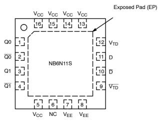
Figure 3. NB6N11S Pinout, 16-pin QFN (Top View)
