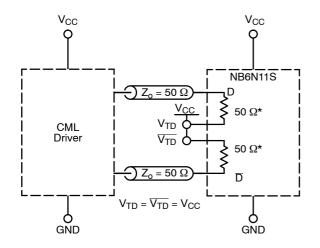
Figure 13. Standard 50  $\Omega$  Load CML Interface
