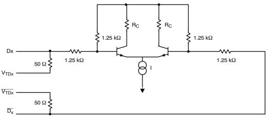
Figure 10. Input Structure
