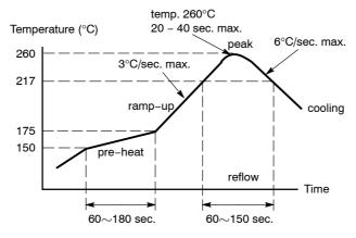
Figure 6. Recommended Reflow Soldering Profile
