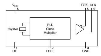
Figure 1. Simplified Logic Diagram
