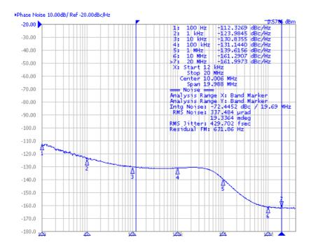
Figure 3. Typical Phase Noise Plot at 106.25 MHz
