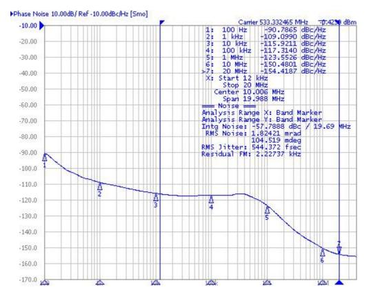
Figure 3. Typical Phase Noise Plot
