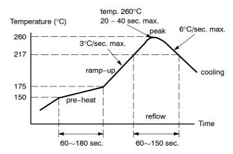
Figure 5. Recommended Reflow Soldering Profile
