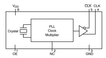
Figure 1. Simplified Logic Diagram
