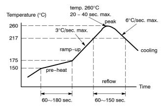
Figure 5. Recommended Reflow Soldering Profile
