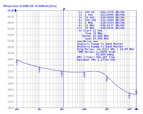
Figure 3. Typical Phase Noise Plot
