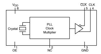
Figure 1. Simplified Logic Diagram
