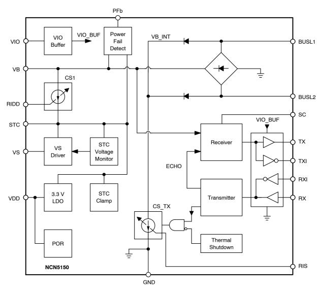
Figure 2. NCN5150 Block Diagram
