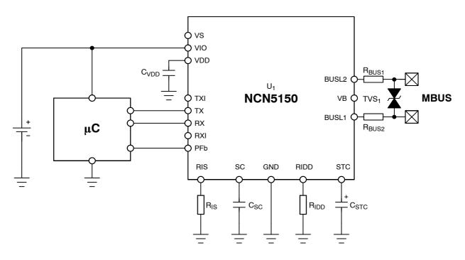
Figure 4. Application Schematic with External Power Supply (Battery)
