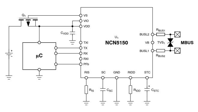
Figure 5. Application Schematic with Backup External Power Supply
