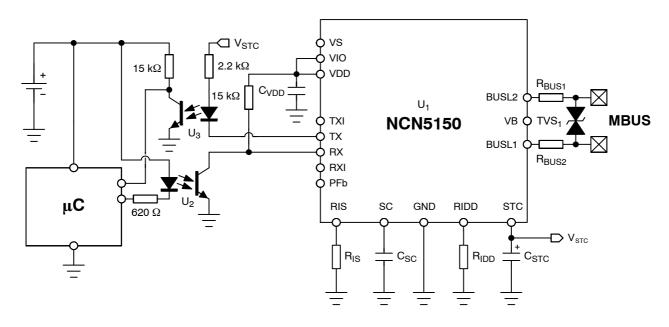
Figure 6. Optically Isolated Application Schematic
