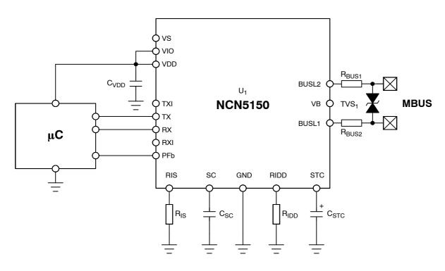
Figure 3. General Application Schematic
