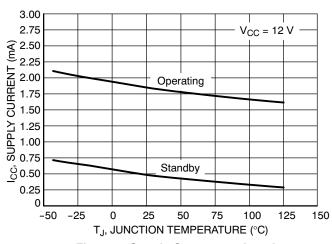
Figure 3. Supply Current vs. Junction Temperature
