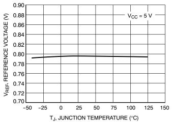
Figure 11. Reference Voltage vs. Junction Temperature
