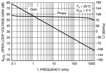
Figure 5. Error Amplifier Open Loop Voltage Gain/Phase vs. Frequency
