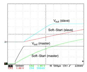
Figure 13. Power-up Sequencing Waveforms
