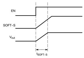
Figure 12. Relationship Between Enable and Soft-Start
