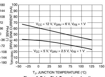
Figure 6. Drive Sink Current vs. Junction Temperature
