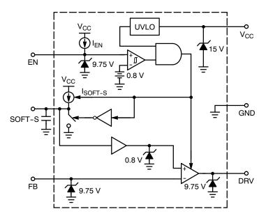
Figure 2. Representative Block Diagram
