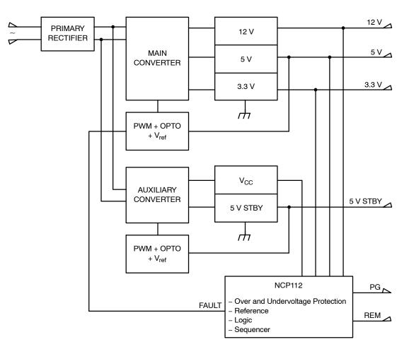
Figure 3. Simplified Application Schematic
