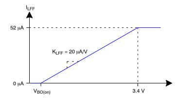
Figure 46. Transfer Function of the Line Feed Forward
