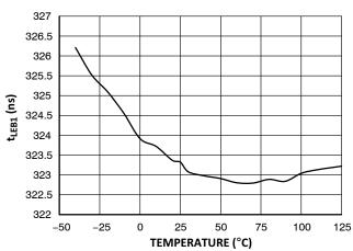
Figure 10.  $t_{\text{LEB1}}$  vs. Junction Temperature
