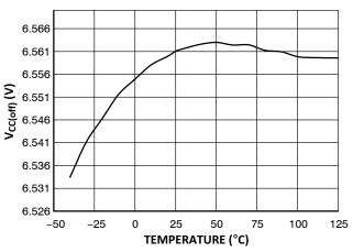
Figure 6.  $V_{\text{CC(off)}}$  vs. Junction Temperature
