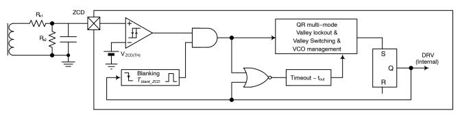
Figure 36. Valley Lockout Detection Circuitry Internal Schematic
