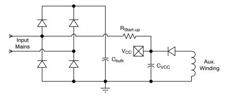
Figure 31. The Startup Resistor can be Connected to the Input Mains for Further Power Dissipation Reduction
