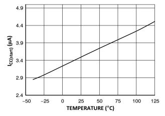
Figure 8. I<sub>CC(start)</sub> vs. Junction Temperature
