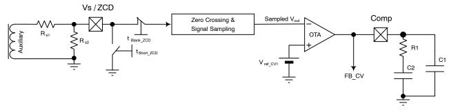
Figure 34. Constant Voltage Feedback Arrangement
