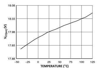
Figure 5. V<sub>CC(on)</sub> vs. Junction Temperature
