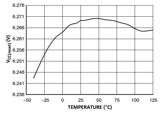
Figure 7. V<sub>CC(reset)</sub> vs. Junction Temperature
