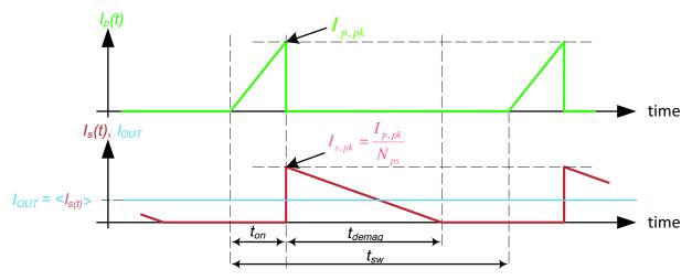
Figure 32. Primary and Secondary Transformer Current Waveforms
