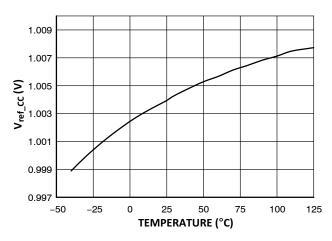
Figure 15.  $V_{ref\_CC}$  vs. Junction Temperature
