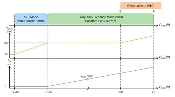
Figure 39. Frequency Foldback and Stanby Mode Behavior with 1-kHz Minimum Frequency Clamp,  $V_{CS(VCO)} = 250 \text{ mV}$  and  $V_{CS(STB)} = 65 \text{ mV}$
