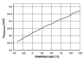
Figure 18. V<sub>ZCD(short)</sub> vs. Junction Temperature
