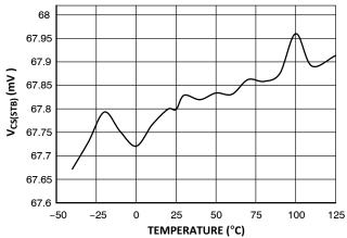
Figure 14.  $V_{CS(STB)}$  vs. Junction Temperature
