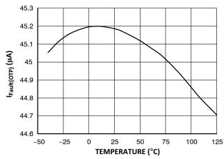
Figure 27. V<sub>Fault(OTP)</sub> vs. Junction Temperature
