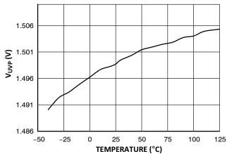
Figure 20.  $V_{\mbox{UVP}}$  vs. Junction Temperature
