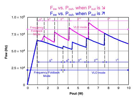
Figure 37. Typical Switching Frequency vs. Output Power Relationship in a 10-W Adapter
