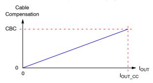
Figure 30. Cable Compensation vs. Output Current Load
