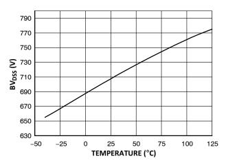
Figure 3. BV<sub>DSS</sub> vs. Junction Temperature
