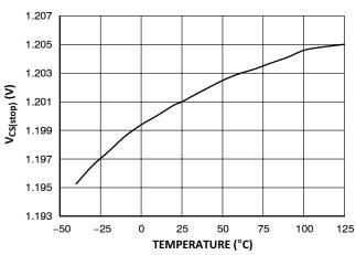
Figure 12. V<sub>CS(stop)</sub> vs. Junction Temperature
