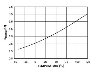
Figure 4. R<sub>DS(on)</sub> vs. Junction Temperature
