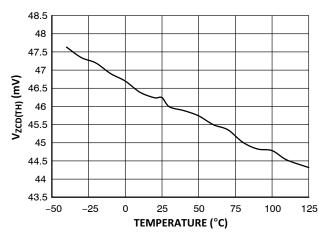
Figure 17.  $V_{\text{ZCD(TH)}}$  vs. Junction Temperature
