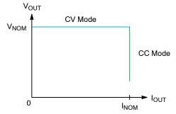
Figure 29. Constant-Voltage & Constant-Current Mode
