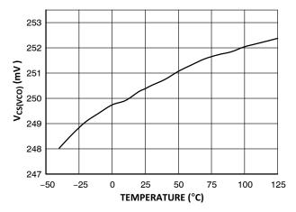
Figure 13.  $V_{CC(VCO)}$  vs. Junction Temperature
