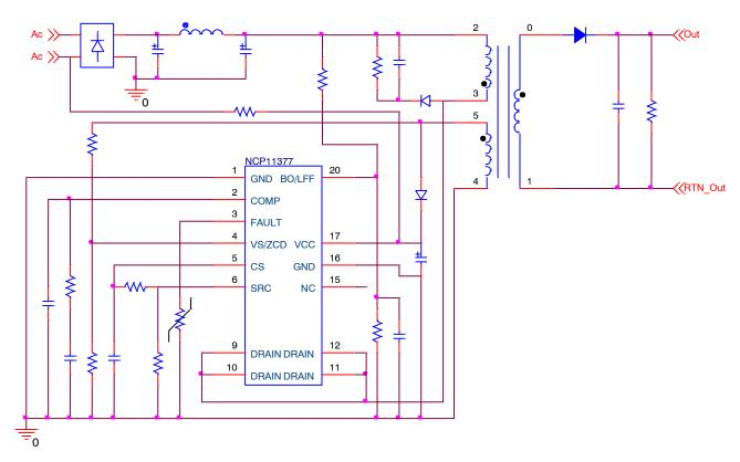
Figure 1. NCP11377 Application Schematic Diagram
