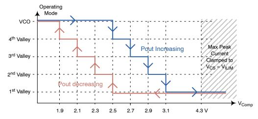
Figure 38. Valley Lockout Threshold
