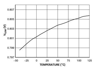
Figure 9.  $V_{\text{ILIM}}$  vs. Junction Temperature
