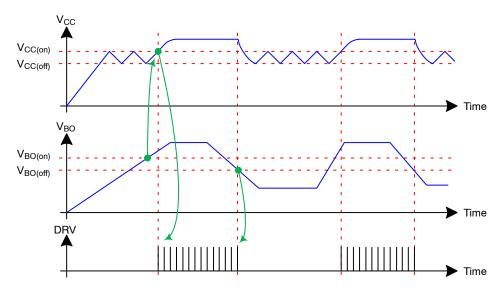
Figure 43. Brown-out Input Functionality –  $V_{CC}$  <  $V_{CC(on)}$
