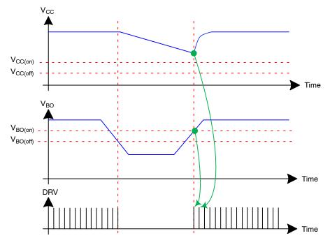
Figure 44. Brown-out Input Functionality –  $V_{CC} > V_{CC(on)}$
