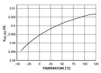
Figure 16.  $V_{ref\_CV1}$  vs. Junction Temperature
