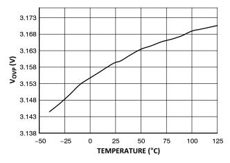
Figure 19.  $V_{\mbox{\scriptsize OVP}}$  vs. Junction Temperature
