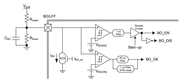
Figure 42. Internal Brown-out Configuration
