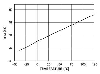
Figure 11. t<sub>ILIM</sub> vs. Junction Temperature
