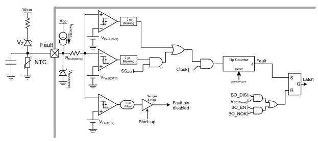
Figure 48. Fault Detection Schematic
