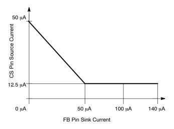
Figure 16. Current Sense Regulation Characteristic
