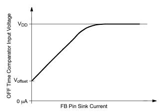
Figure 14. FB Loop Transfer Characteristic
