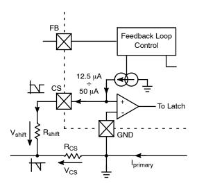
Figure 19. Primary Current Sensing
