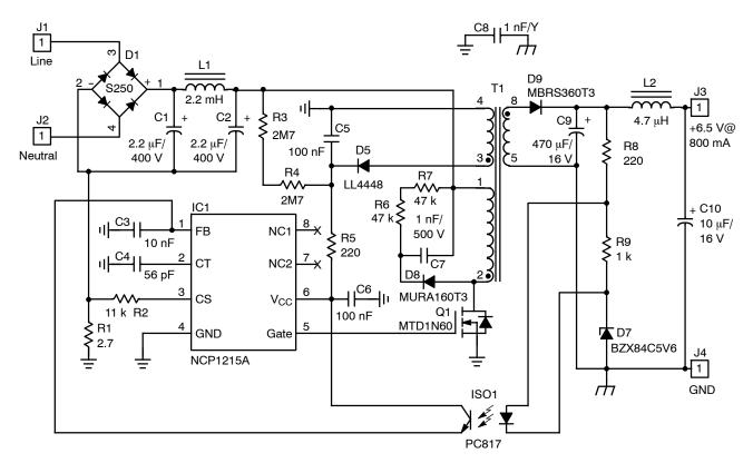
Figure 21. Adaptor Application Schematic
