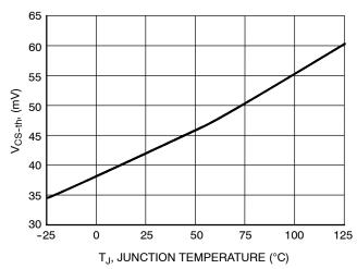
Figure 7. Current Sense Source Current vs. Junction Temperature
