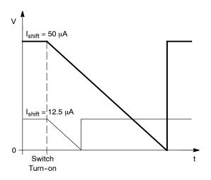
Figure 20. CS Pin Voltage
