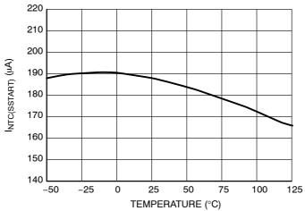
Figure 29. Current  $I_{\mbox{NTC}(\mbox{SSTART})}$  Sourced from the Latch Pin, During Soft-Start
