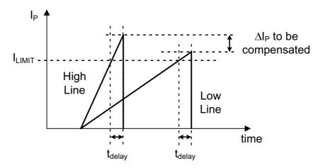
Figure 38. Line Compensation for True Overpower Protection
