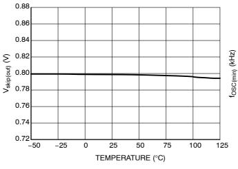
Figure 19. FB Pin Skip-Out Level V<sub>skip(out)</sub>
