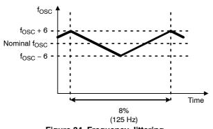
Figure 34. Frequency Jittering
