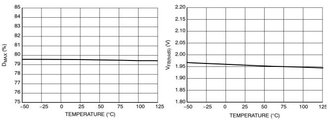
Figure 15. Maximum Duty Cycle D<sub>MAX</sub>
