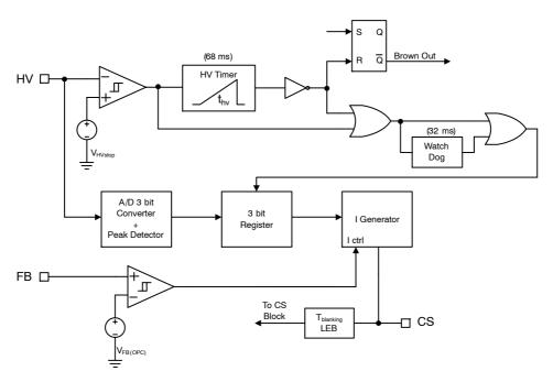
Figure 39. Schematic Overpower Compensation Circuit
