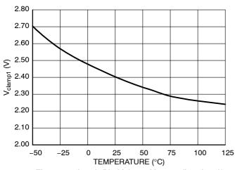
Figure 27. Latch Pin Voltage V<sub>clamp1</sub> (Latch-off Pin is Sinking 1 mA)
