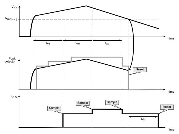
Figure 42. Overpower Compensation
