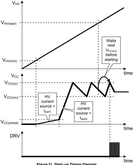
Figure 31. Start-up Timing Diagram
