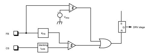
Figure 48. Skip Cycle Schematic
