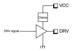
Figure 35. Clamped Driver
