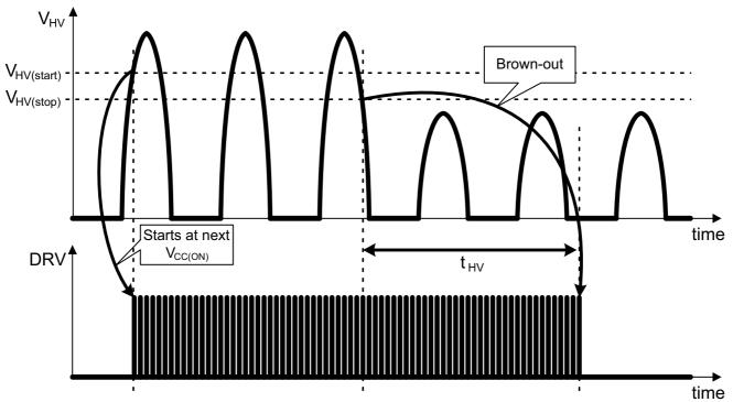
Figure 33. AC Input Brown-out Timing Diagram
