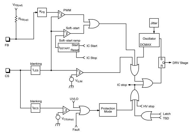
Figure 36. Current Sense Block Schematic
