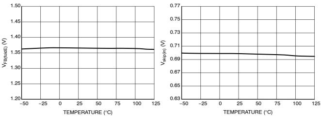
Figure 17. FB Pin Voltage Below Which Frequency Foldback is Complete V<sub>FB(foldE)</sub>
