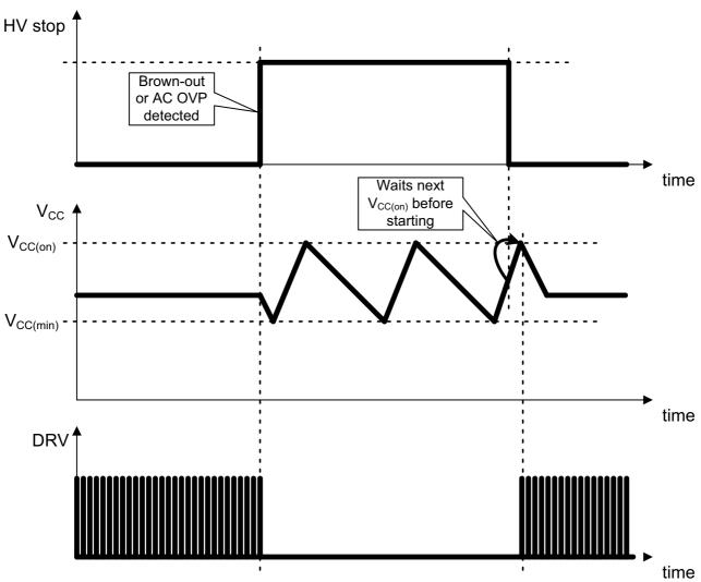
Figure 32. Brown-out Timing Diagram
