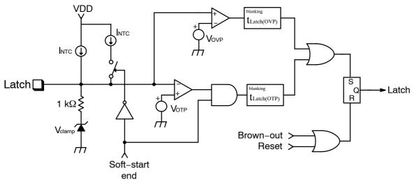
Figure 50. Latch Detection Schematic
