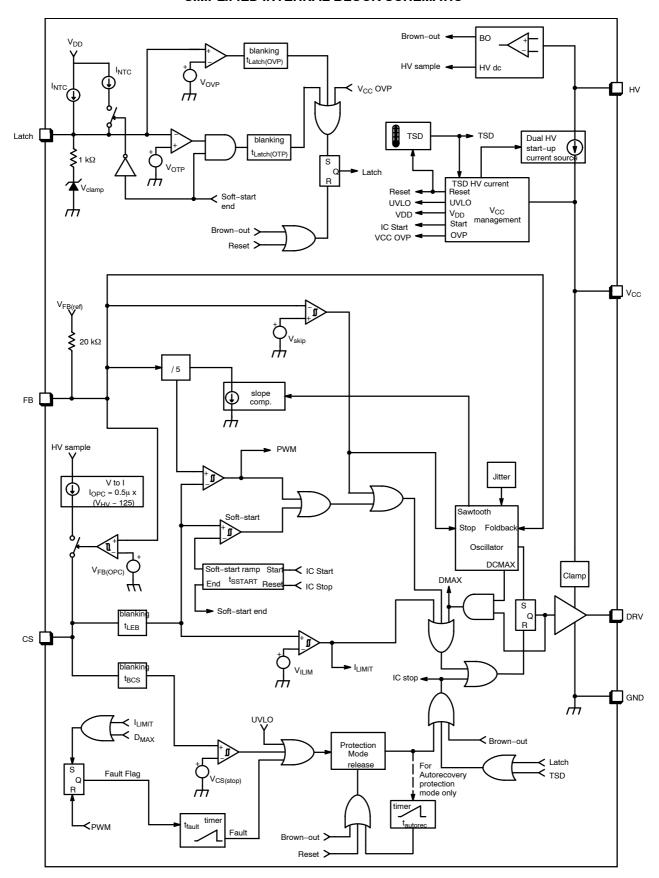
Figure 2. Simplified Internal Block Schematic
