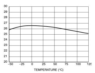
Figure 20. Minimum Switching Frequency f<sub>OSC(min)</sub>
