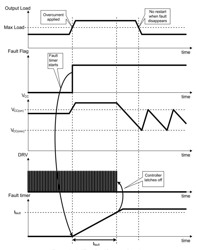
Figure 46. Latched Timer-Based Overcurrent Protection
