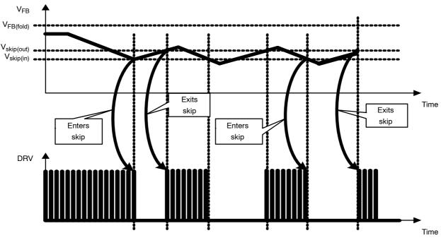
Figure 49. Skip Cycle Timing Diagram
