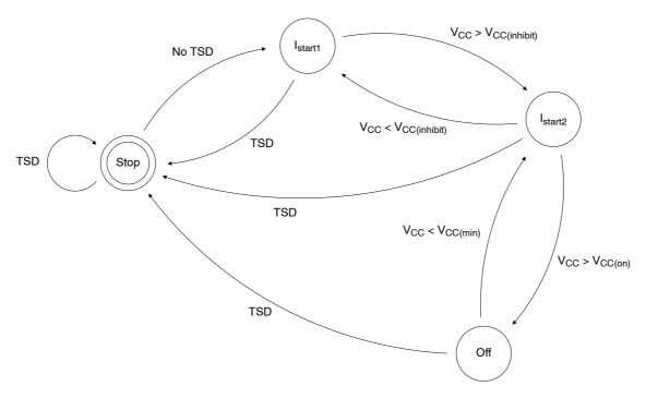
Figure 52. HV Start-up Current Source State Diagram
