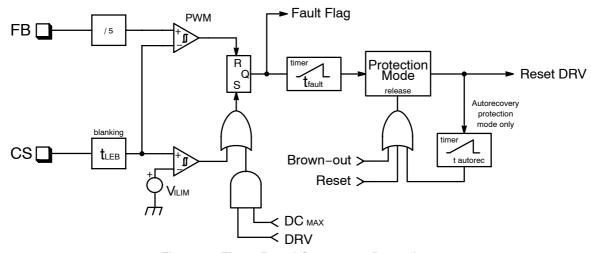
Figure 44. Timer-Based Overcurrent Protection
