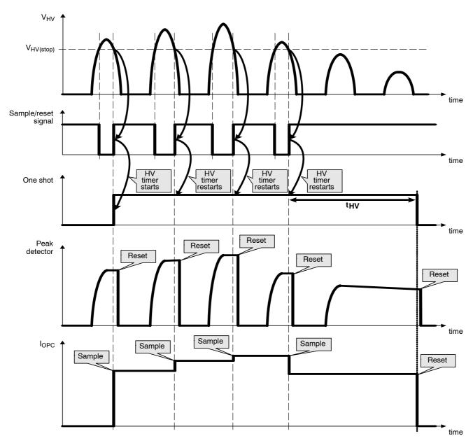
Figure 41. Overpower Compensation
