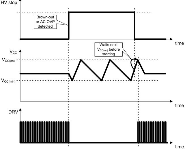
Figure 43. Brown-out or Line Overvoltage Timing Diagram
