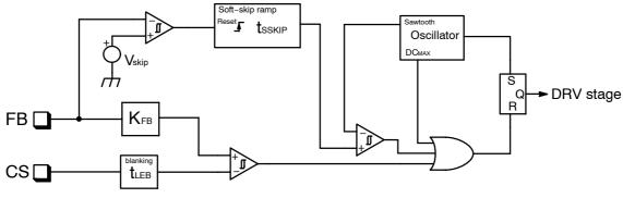
Figure 60. Skip Cycle with Soft-Skip Schematic
