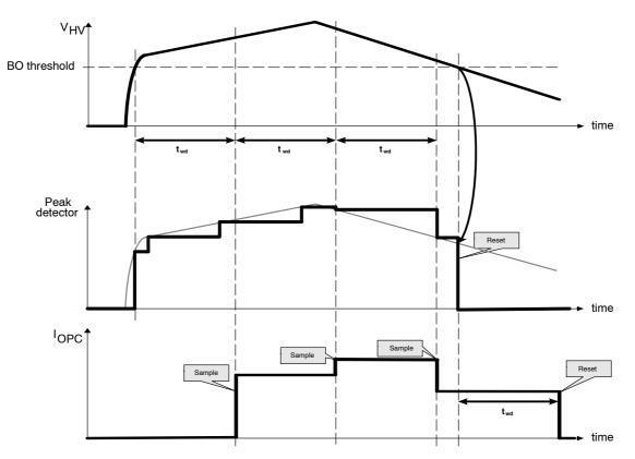
Figure 54. Overpower Compensation Current with the HV pin connected to a dc voltage
