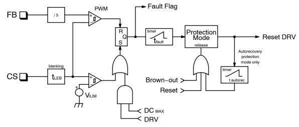
Figure 56. Timer-Based Overcurrent Protection
