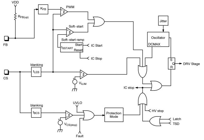
Figure 48. Current Sense Block Schematic
