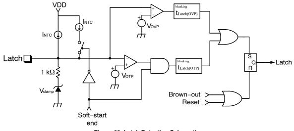
Figure 62. Latch Detection Schematic
