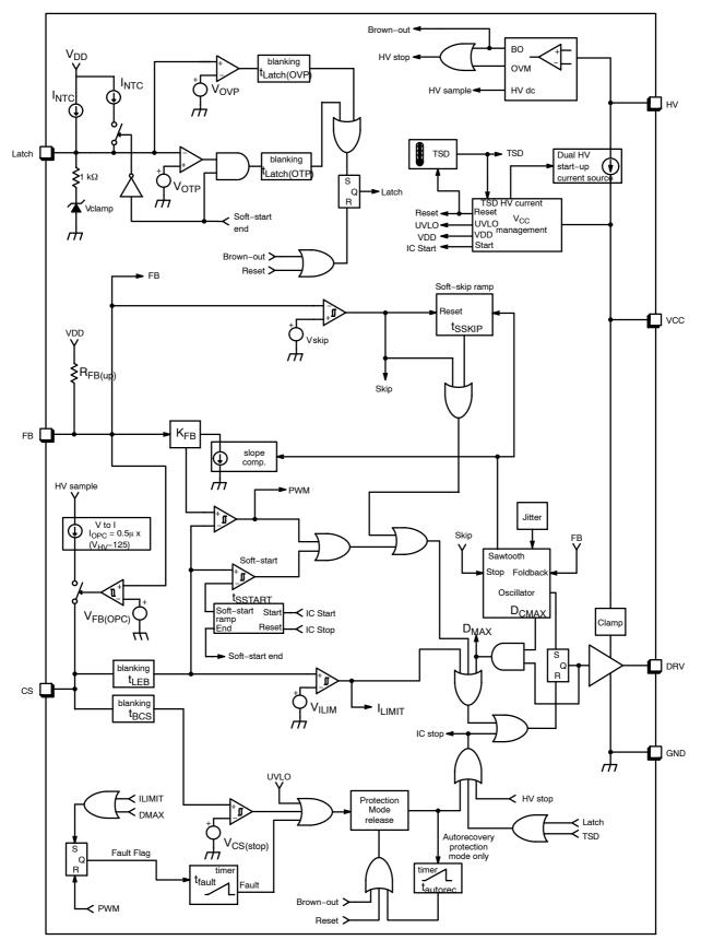
Figure 3. Simplified Internal Block Schematic
