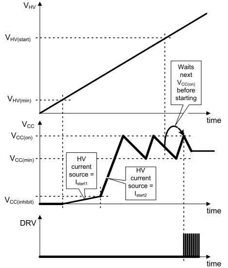
Figure 42. Startup Timing Diagram
