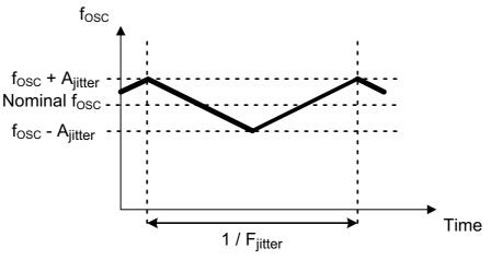
Figure 46. Frequency Jittering
