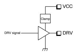
Figure 47. Clamped Driver
