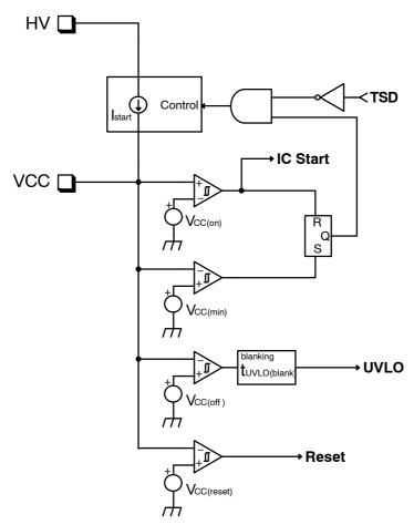
Figure 41. HV Startup Current Source Functional Schematic
