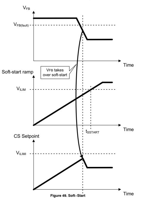
Under some conditions, like a winding short-circuit for instance, not all the energy stored during the *on* time is transferred to the output during the *off* time, even if the on time duration is at its minimum (imposed by the propagation delay of the detector added to the LEB duration). As a result, the current sense voltage keeps on increasing above  $V_{ILIM}$ , because the controller is blind during the LEB blanking
