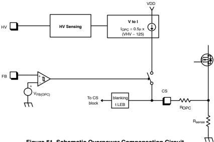
Figure 51. Schematic Overpower Compensation Circuit
