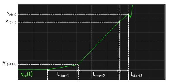
Figure 32. The  $V_{CC}$  at Start-Up is Made of Two Segments Given the Short-Circuit Protection Implemented on the HV Source
