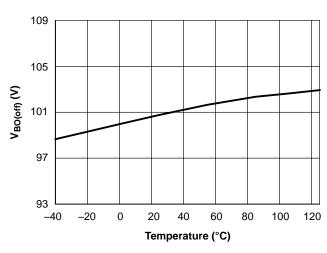
Figure 24. V<sub>BO(off)</sub> vs. Junction Temperature
