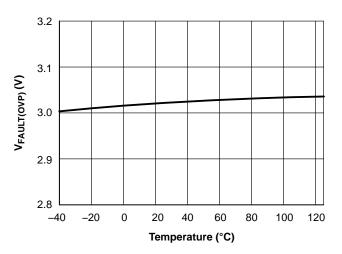
Figure 26. V<sub>FAULT(OVP)</sub> vs. Junction Temperature
