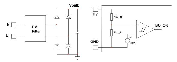
Figure 33. A Simplified View of the Brown-Out Circuitry
