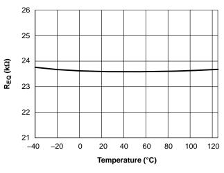
Figure 21.  $R_{EQ}$  vs. Junction Temperature
