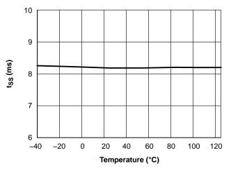
Figure 17. t<sub>SS</sub> vs. Junction Temperature
