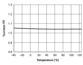
Figure 30. t<sub>AUTOREC</sub> vs. Junction Temperature
