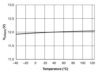
Figure 3. V<sub>CC(on)</sub> vs. Junction Temperature
