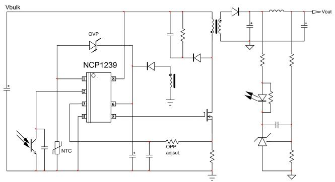
Figure 1. Application Schematic (OPP Adjustment)
