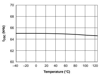
Figure 18. f<sub>OSC</sub> (65-kHz Version) vs. Junction Temperature
