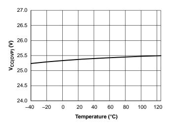
Figure 31. V<sub>CC(OVP)</sub> vs. Junction Temperature
