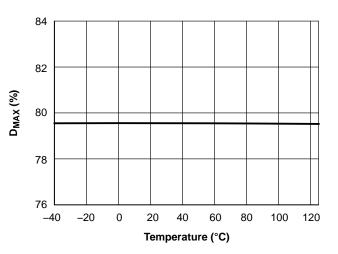
Figure 20. D<sub>MAX</sub> vs. Junction Temperature
