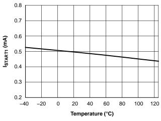
Figure 9. I<sub>START1</sub> vs. Junction Temperature
