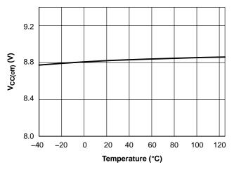
Figure 5. V<sub>CC(off)</sub> vs. Junction Temperature
