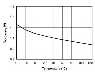
Figure 6. V<sub>CC(inhibit)</sub> vs. Junction Temperature
