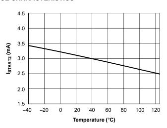
Figure 10. I<sub>START2</sub> vs. Junction Temperature
