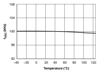
Figure 19. f<sub>OSC</sub> (100-kHz Version) vs. Junction Temperature
