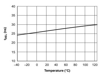
Figure 14. t<sub>DEL</sub> vs. Junction Temperature
