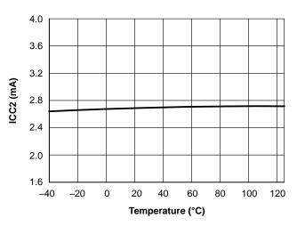
Figure 8. ICC2 (100-kHz Version) vs. Junction Temperature
