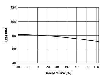
Figure 16. t<sub>LEB2</sub> vs. Junction Temperature
