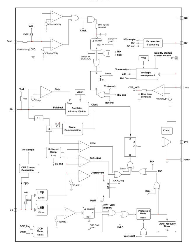
Figure 2. Simplified Block Diagram
