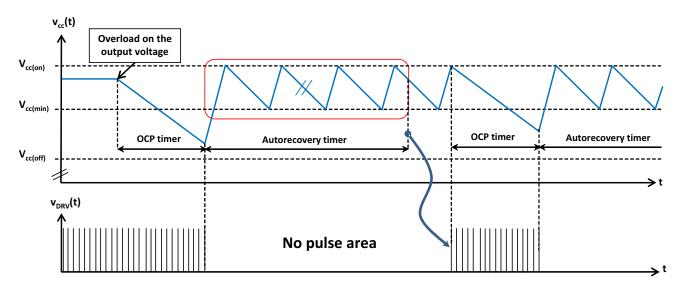
Figure 39. An Auto-Recovery Hiccup Mode is Entered in Case a Faulty Event Longer than 64 ms is Acknowledged by the Controller
