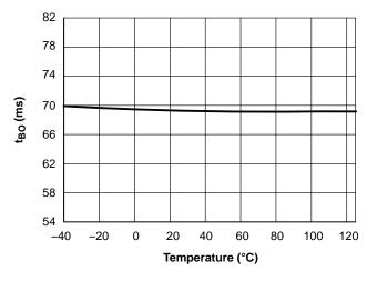
Figure 25. t<sub>BO</sub> vs. Junction Temperature
