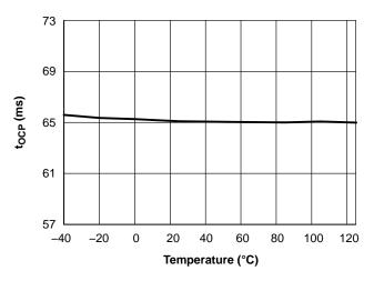
Figure 29. t<sub>OCP</sub> vs. Junction Temperature
