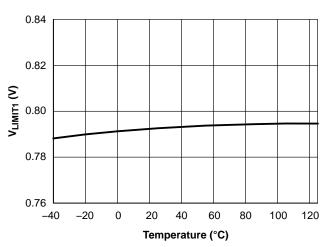
Figure 12. V<sub>LIMIT1</sub> vs. Junction Temperature
