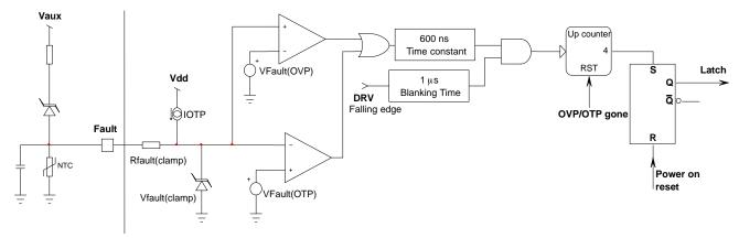
Figure 38. Fault Detection Schematic
