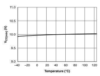
Figure 4. V<sub>CC(min)</sub> vs. Junction Temperature
