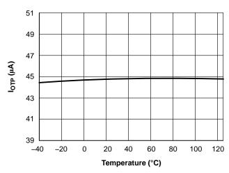
Figure 28. I<sub>OTP</sub> vs. Junction Temperature
