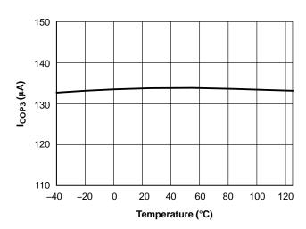
Figure 22. I<sub>OOP3</sub> vs. Junction Temperature
