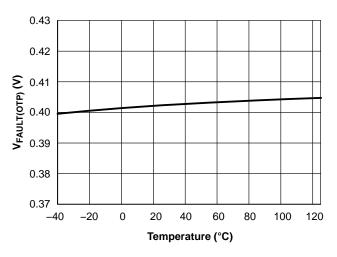
Figure 27. V<sub>FAULT(OTP)</sub> vs. Junction Temperature
