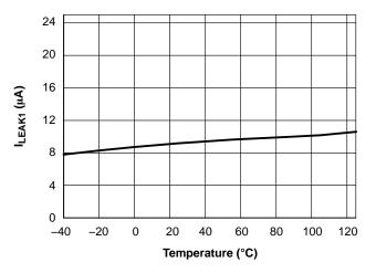
Figure 11. I<sub>LEAK1</sub> vs. Junction Temperature
