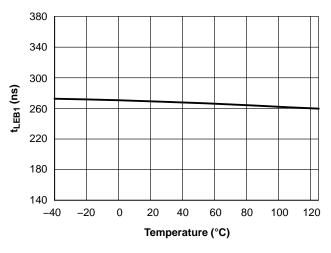
Figure 15. t<sub>LEB1</sub> vs. Junction Temperature
