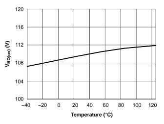
Figure 23. V<sub>BO(on)</sub> vs. Junction Temperature
