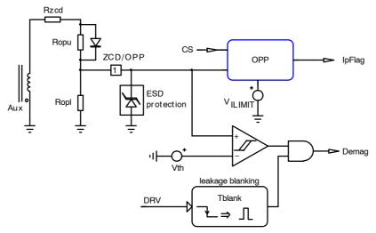
Figure 35. Over Power Compensation Circuit
