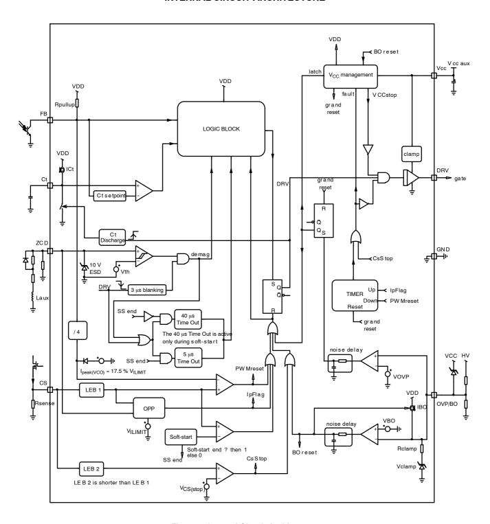
Figure 2. Internal Circuit Architecture
