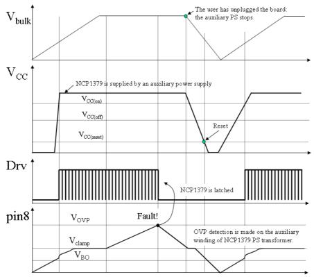
Figure 37. Operating Chronograms in Case of Overvoltage with NCP1379 Supplied by an Auxiliary Power Supply
