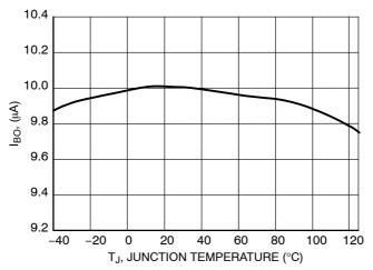
Figure 21. I<sub>BO</sub> vs. Junction Temperature
