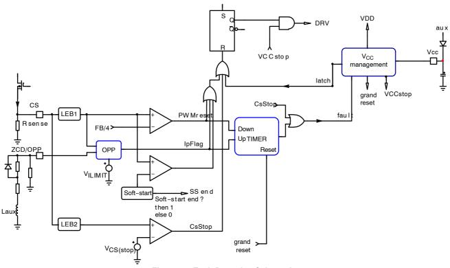
Figure 33. Fault Detection Schematic
