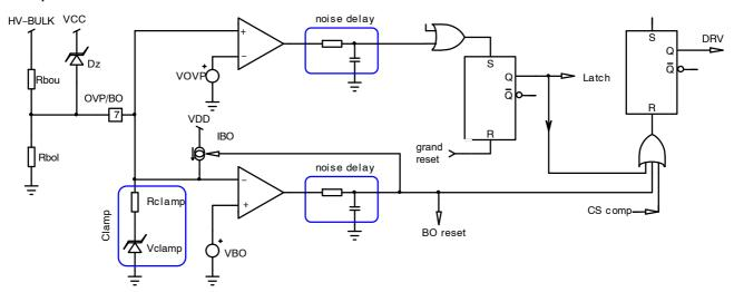
Figure 36. Brown-out and Overvoltage Protection
