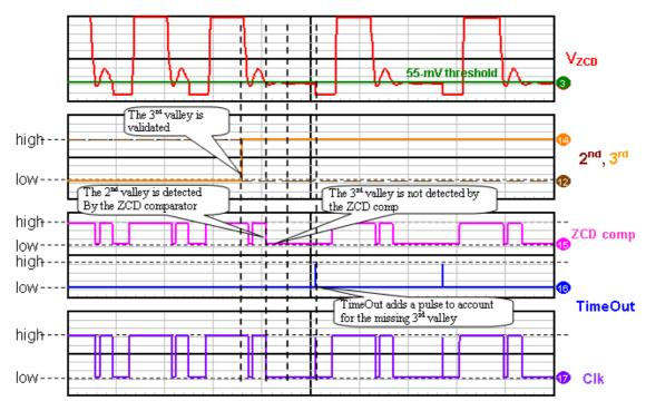
Figure 30. Time Out Case n°1: the 3<sup>rd</sup> Valley is Missing
