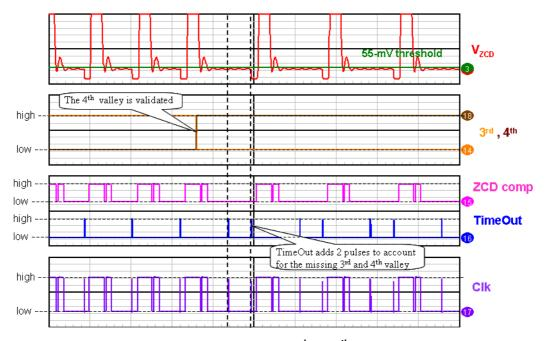
Figure 31. Time Out Case n°2: the 3<sup>rd</sup> and 4<sup>th</sup> Valley are Missing
