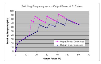
Figure 11. Switching Frequency Evolution versus Output Power at V<sub>in</sub> = 115 Vrms
