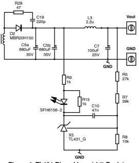
Figure 4. TL431 Biased by a 1  $k\Omega$  Resistor
