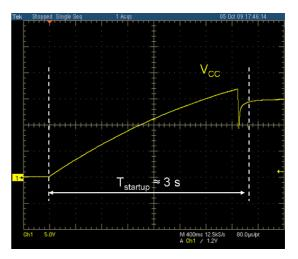
Figure 15. Startup Duration with a 1.3 M $\Omega$  Resistor Connected to the Half–Wave, V<sub>in</sub> = 85 Vrms
