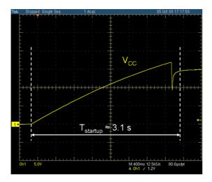
Figure 14. Startup Duration with a 3.2 M $\Omega$  Resistor Connected to the Bulk Rail, V<sub>in</sub> = 85 Vrms
