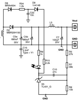
Figure 5. TL431 Bias Removal Circuit
