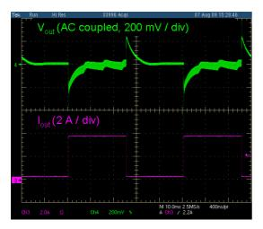
Figure 16. Transient Load Step Response at V<sub>in</sub> = 115 Vrms
