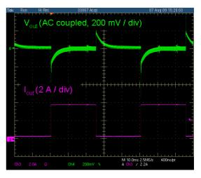
Figure 17. Transient Load Step Response at V<sub>in</sub> = 230 Vrms
