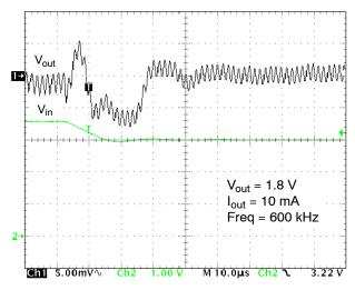
Figure 27. Line Transient from 3.6 to 3.0 V
