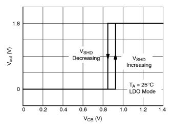
Figure 17. Output Voltage versus Shutdown
