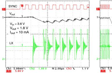
Figure 24. Transition from LDO to PWM Mode
