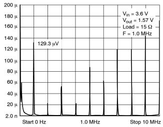
Figure 30. V<sub>rms</sub> versus Frequency
