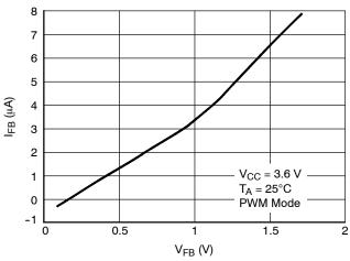
Figure 13. Input Current versus Voltage for the Feedback Pin
