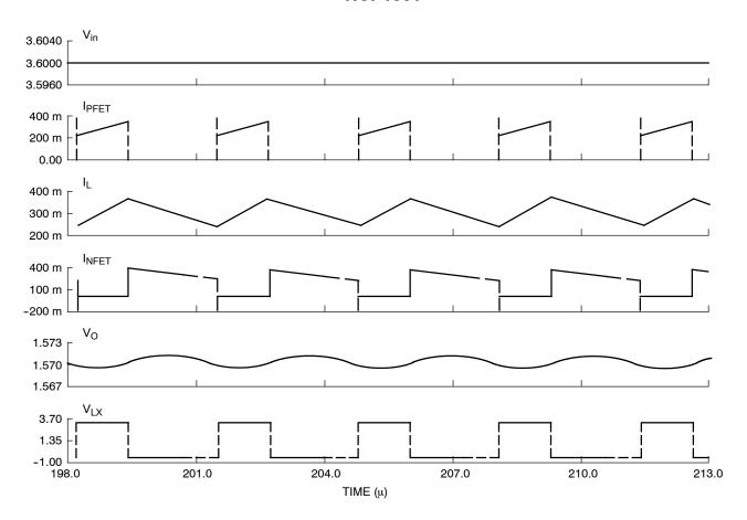
Figure 8. Waveforms During Normal Operation
