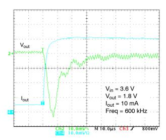
Figure 28. Load Transient from 10 to 100 mA
