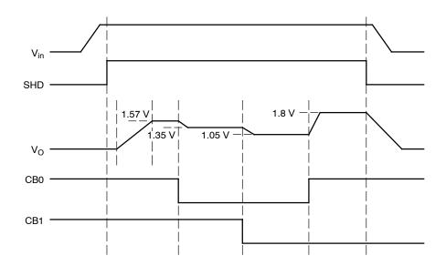
Figure 7. Power Up and Power Down Sequence
