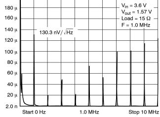
Figure 32. Noise versus Frequency
