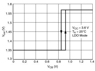
Figure 15. Transition Level of CB Pins
