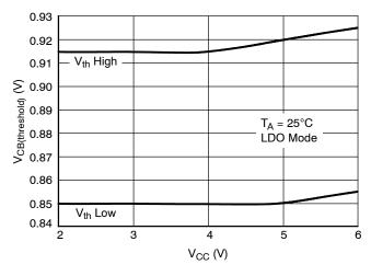
Figure 14. V<sub>CC</sub> Input Voltage versus CB Threshold
