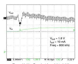
Figure 26. Line Transient from 3.0 to 3.6 V
