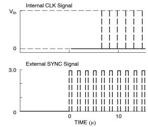
Figure 6. Transition Waveforms from LDO to PWM Mode
