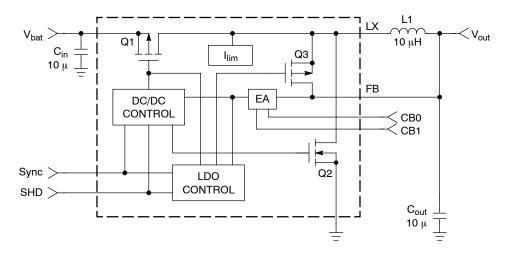
Figure 3. Block Diagram and Circuit Schematic of the NCP1501
