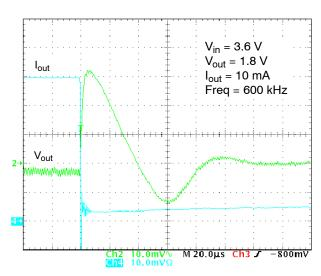
Figure 29. Load Transient from 100 to 10 mA
