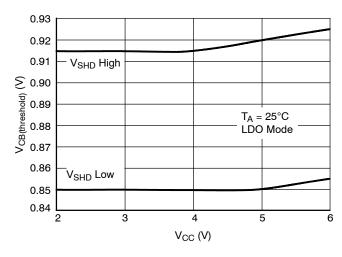
Figure 16. Input Voltage versus Shutdown Voltage
