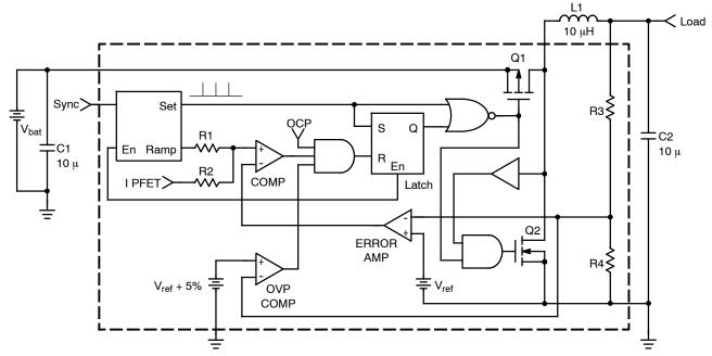
Figure 4. PWM Circuit Schematic
