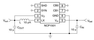
Figure 1. Typical Applications Circuit
