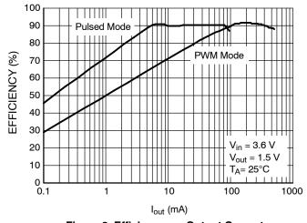
Figure 2. Efficiency vs. Output Current
