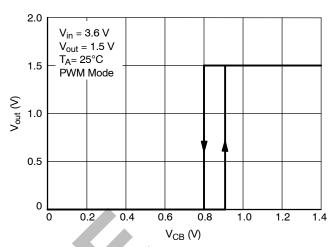
Figure 17. Transition Level of CB Pins
