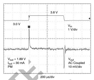
Figure 23. Line Transient Response for PM
