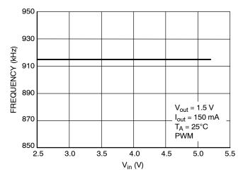
Figure 15. Oscillator Frequency vs. Input Voltage
