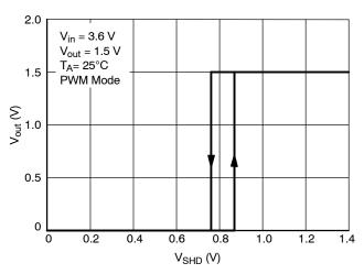
Figure 16. Output Voltage vs. Shutdown Pin Voltage
