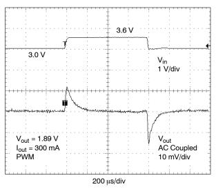
Figure 22. Line Transient Response for PWM
