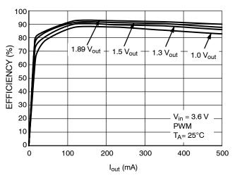
Figure 4. Efficiency vs. Output Current in PWM Mode
