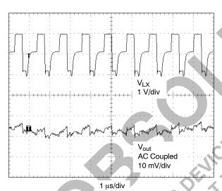
Figure 18. Light Load PWM Switching Waveform (V<sub>in</sub> = 3.6 V, V<sub>out</sub> = 1.5 V, I<sub>out</sub> = 30 mA)
