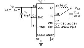
Figure 1. Typical Application Circuit
