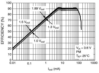
Figure 9. Efficiency vs. Output Current in Pulsed Mode
