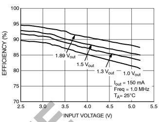
Figure 5. Efficiency vs. Input Voltage in PWM Mode
