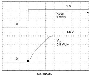
Figure 21. Soft-Start (V<sub>in</sub> = 3.6 V, V<sub>out</sub> = 1.5 V, I<sub>out</sub> = 150 mA)
