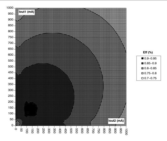
Figure 3. Efficiency vs. Output Current ( $V_{IN}$  = 3.6 V,  $V_{OUT1}$  = 1.8 V,  $V_{OUT2}$  = 1.8 V, Temperature = 25°C) MODE/SYNC Pin = GND
