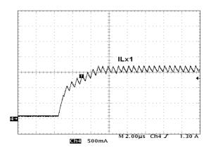
Figure 19. Current Peak Inductor Protection  $V_{IN}$  = 3.6 V,  $V_{OUT1}$  = 1.2 V,  $I_{OUT1}$  Short to GND, EN2 = GND
