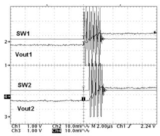
Figure 23. PFM Switching Waveforms  $V_{IN}$  = 3.6 V,  $V_{OUT1}$  =  $V_{OUT2}$  = 1.2 V,  $I_{OUT1}$  =  $I_{OUT2}$  = 0 mA
