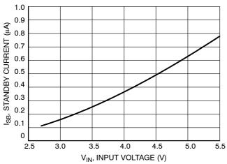
Figure 10. Standby Current vs. Input Voltage V<sub>IN</sub> = 3.6 V, EN1 = EN2 = GND, Temperature = 25°C
