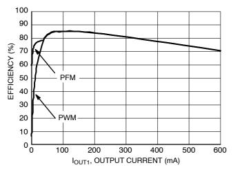
Figure 4. Efficiency vs. Output Current  $V_{IN}$  = 3.6 V,  $V_{OUT1}$  = 1.2 V, EN2 = GND
