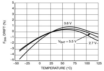
Figure 16. Switching Frequency vs.
