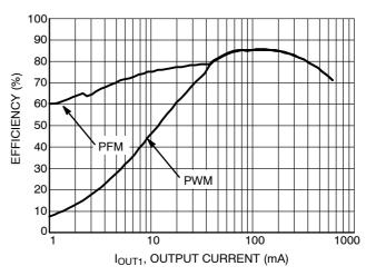
Figure 5. Efficiency vs. Output Current  $V_{IN} = 3.6 \text{ V}$ ,  $V_{OUT1} = 1.2 \text{ V}$ , EN2 = GND
