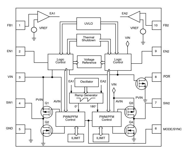
Figure 2. Simplified Block Diagram
