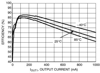
Figure 6. Efficiency vs. Output Current  $V_{IN}$  = 3.6 V,  $V_{OUT1}$  = 1.2 V, EN2 = GND, Temperature = 25°C
