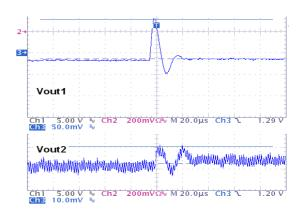
Figure 15. Load Transient and Crosstalk,
