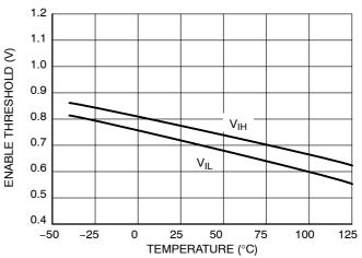
Figure 21. Enable Thresholds  $V_{IN}$  = 3.6 V,  $I_{OUT1}$  =  $I_{OUT2}$  = 2 mA
