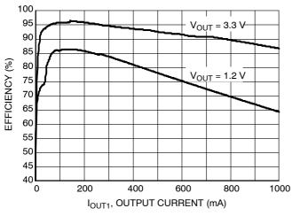
Figure 8. Efficiency vs. Output Current  $V_{IN}$  = 3.6 V, EN2 = GND, Temperature = 25°C
