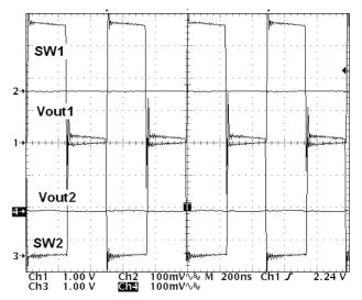
Figure 22. PWM Switching Waveforms  $V_{IN} = 3.6 \text{ V}$ ,  $V_{OUT1} = V_{OUT2} = 1.2 \text{ V}$ ,  $I_{OUT1} = I_{OUT2} = 100 \text{ mA}$
