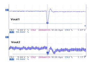
Figure 14. Load Transient and Crosstalk,  $V_{IN}$  = 3.6 V  $V_{OUT1}$  = 1.2 V,  $I_{OUT1}$  from 200 mA to 600 mA  $V_{OUT2}$  = 1.2 V,  $I_{OUT2}$  = 600 mA, 8 mV Crosstalk
