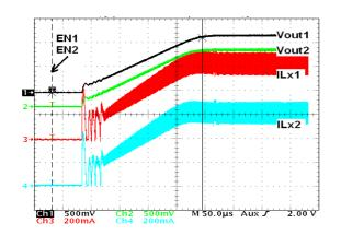
Figure 18. Soft-Start Typical Behavior  $V_{IN}$  = 3.6 V,  $V_{OUT1}$  =  $V_{OUT2}$  = 1.2 V,  $I_{OUT1}$  =  $I_{OUT2}$  = 600 mA
