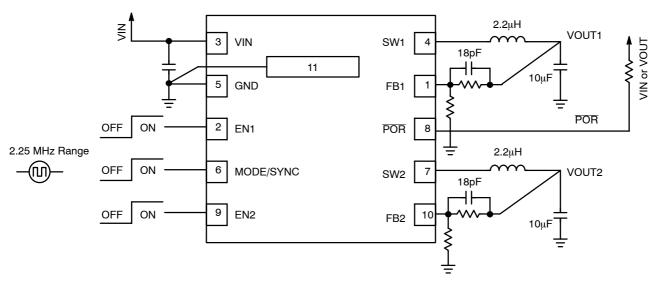
NOTE: Exposed pad of UDFN10 package - named pin11 - must be connected to system ground.
