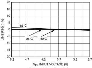
Figure 12. Line Regulation V<sub>OUT1</sub> = 1.2 V, I<sub>OUT1</sub> = 100 mA, EN2 = GND
