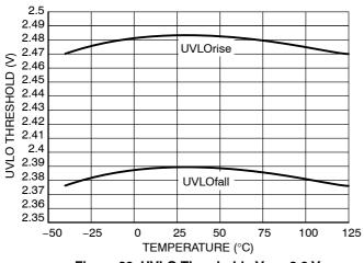
Figure 20. UVLO Thresholds  $V_{IN}$  = 3.6 V,  $I_{OUT1}$  =  $I_{OUT2}$  = 2 mA
