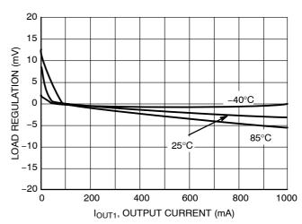
Figure 13. Load Regulation  $V_{IN}$  = 3.6 V,  $V_{OUT1}$  = 1.2 V, EN2 = GND
