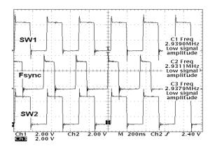
Figure 17. External Synchronization, F<sub>sync</sub> = 2.93 MHz
