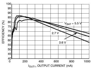
Figure 7. Efficiency vs. Output Current V<sub>OUT1</sub> = 1.2 V, EN2 = GND, Temperature = 25°C
