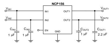
Figure 1. Typical Application Schematic
