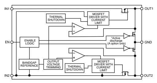
Figure 2. Simplified Schematic Block Diagram
