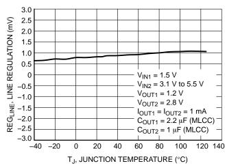
Figure 5. Line Regulation vs. Temperature –  $V_{OUT1} = 1.2 \text{ V}$
