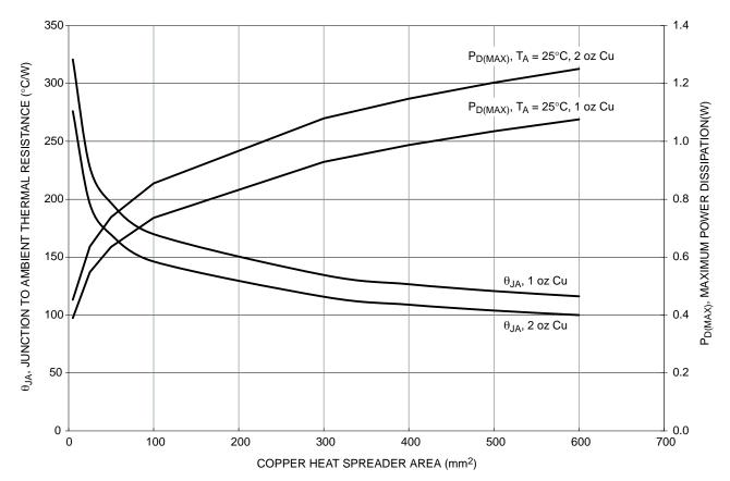
Figure 9.  $\theta_{JA}$  vs. Copper Area (WLCSP-6)
