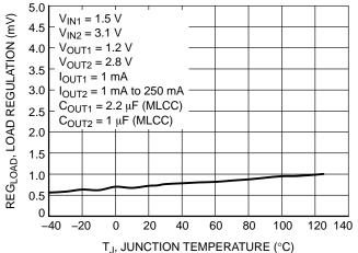
Figure 7. Load Regulation vs. Temperature –  $V_{OUT1} = 1.2 \text{ V}$
