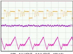
(VIN = 5 V, VOUT = 3.3 V, IOUT = 100 mA) Upper Trace: LX Pin Switching Waveforms, 5 V / div Middle Trace: Output Voltage, 20 mV / div Lower Trace: Inductor Current, 200 mA / div Time = 500 ns / div
