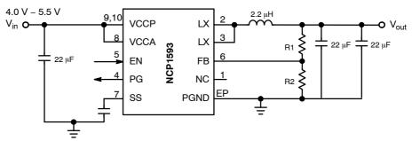
Figure 2. Recommended Application Circuit
