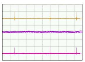
$\begin{array}{l} (\text{VIN}=5 \text{ V}, \text{VOUT}=1.05 \text{ V}, \text{IOUT}=0 \text{ A}) \\ \text{Upper Trace: LX Pin Switching Waveforms, 5 V / div} \\ \text{Middle Trace: Output Voltage, 20 mV / div} \\ \text{Lower Trace: Inductor Current, 100 mA / div} \\ \text{Time}=20 \ \mu \text{s} \ / \ \text{div} \end{array}$
