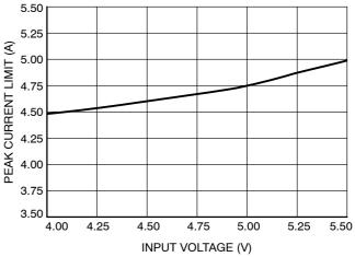
Figure 10. Current Limit vs. Input Voltage
