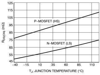
Figure 11. R<sub>DS(ON)</sub> vs. Temperature
