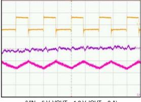
(VIN = 5 V, VOUT = 1.8 V, IOUT = 3 A) Upper Trace: LX Pin Switching Waveforms, 5 V / div Middle Trace: Output Voltage, 20 mV / div Lower Trace: Inductor Current, 2 A / div Time = 500 ns / div
