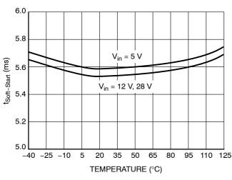
Figure 21. Soft-Start Time vs. Input Voltage and Temperature
