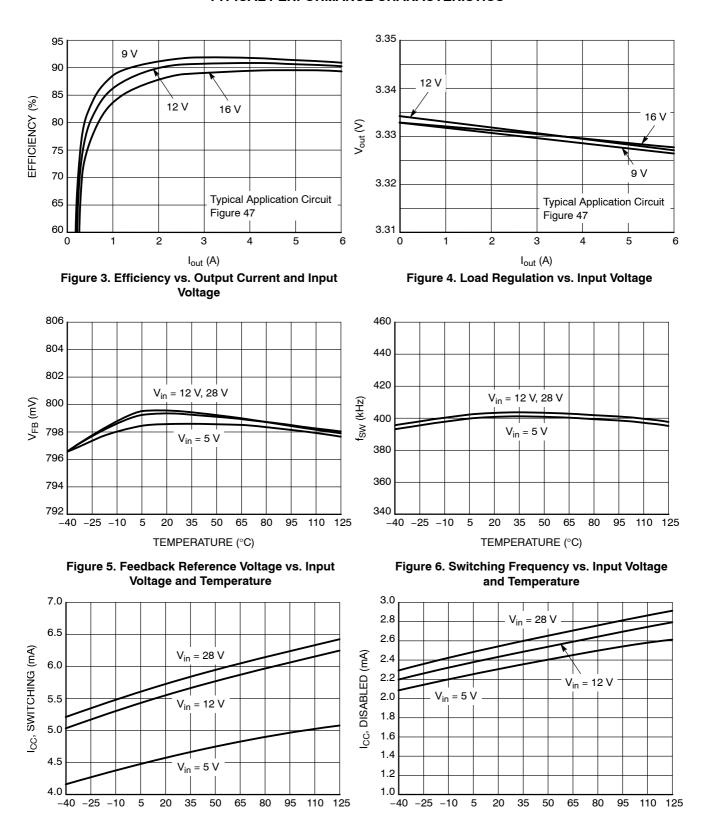
Figure 7. Supply Current vs. Input Voltage and Temperature
