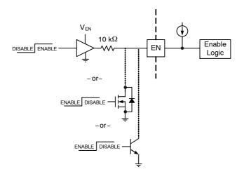
Figure 27. Enable Circuits: Push-Pull, Open-Drain, or Open-Collector
