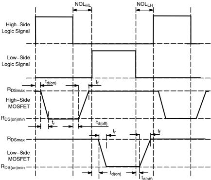
Figure 44. MOSFETs Timing Diagram
