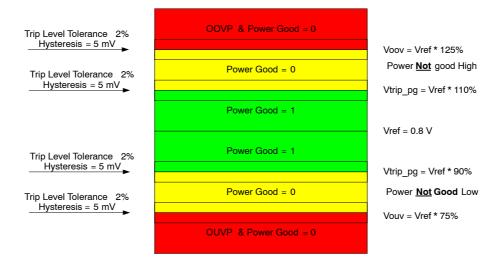
Figure 33. OOV, OUV, and Power Good Window Diagram
