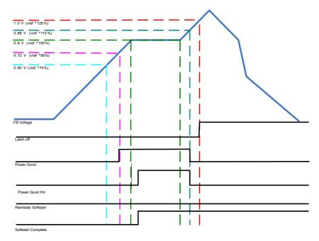
Figure 34. Powerup Sequence and Overvoltage Latch
