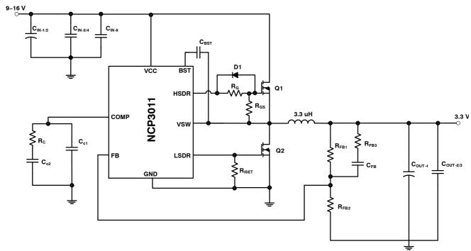
Figure 47. Typical Application,  $V_{\text{IN}}$  = 9 – 16 V,  $V_{\text{OUT}}$  = 3.3 V,  $I_{\text{OUT}}$  = 6 A
