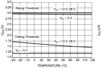
Figure 13. Enable Thresold vs. Input Voltage and Temperature
