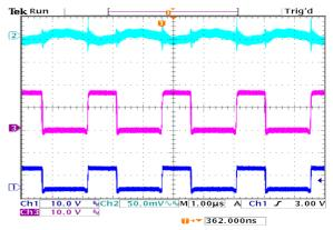
Input = 9 V, Output = 3.3 V, Load = 5 A C1 (Blue) = VSW, C2 (Light Blue) = V<sub>OUT</sub> C3 (Magenta) = HSDR
