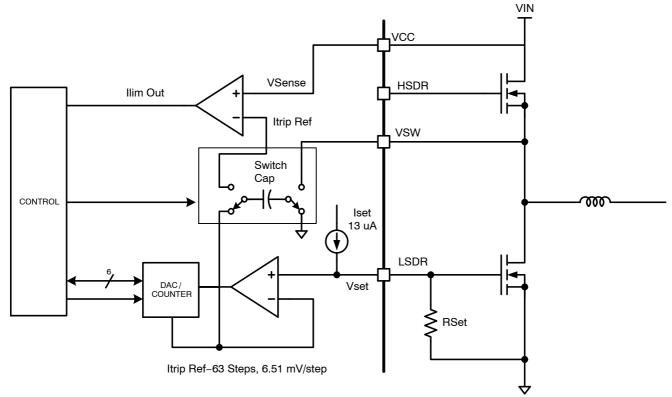
Figure 36. I<sub>set</sub> / I<sub>Limit</sub> Block Diagram
