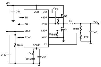
Figure 1. Typical Application Circuit
