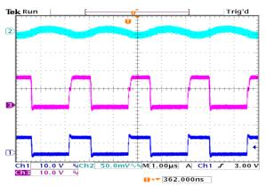
Input = 9 V, Output = 3.3 V, Load = 0 A C1 (Blue) = VSW, C2 (Light Blue) = V<sub>OUT</sub> C3 (Magenta) = HSDR
