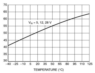
Figure 14. Enable Pullup Current vs. Input Voltage and Temperature
