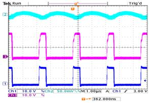
Input = 16 V, Output = 3.3 V, Load = 0 A C1 (Blue) = VSW, C2 (Light Blue) = V<sub>OUT</sub> C3 (Magenta) = HSDR
