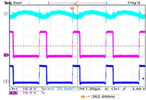
Input = 16 V, Output = 3.3 V, Load = 5 A C1 (Blue) = VSW, C2 (Light Blue) = V<sub>OUT</sub> C3 (Magenta) = HSDR
