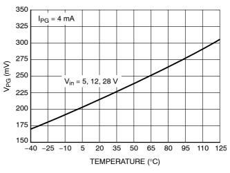
Figure 12. Power Good Output Low Voltage vs. Input Voltage and Temperature
