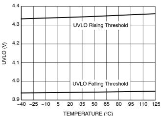
Figure 10. Input Undervoltage Lockout vs.
