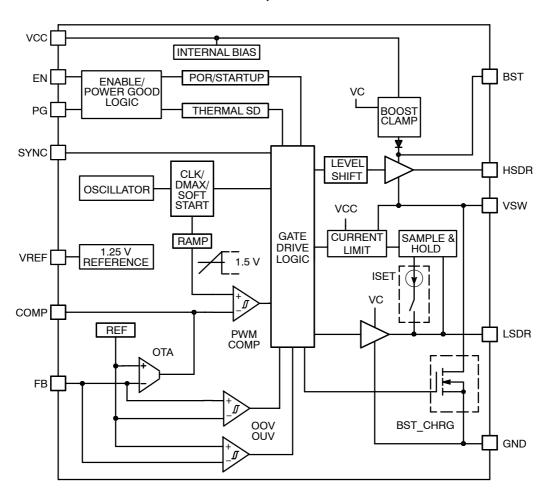
Figure 2. NCP3011 Block Diagram
