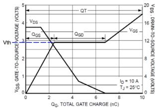
Figure 34. MOSFET Switching Characteristics
