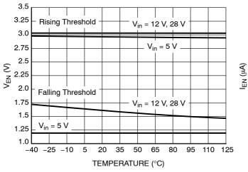
Figure 11. Enable Thresold vs. Input Voltage and Temperature
