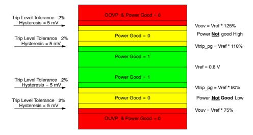
Figure 24. OOV, OUV, and Power Good Window Diagram
