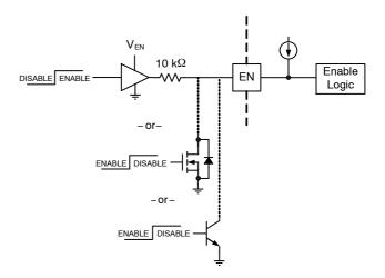
Figure 18. Enable Circuits: Push-Pull, Open-Drain, or Open-Collector
