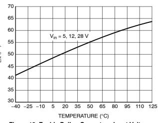
Figure 12. Enable Pullup Current vs. Input Voltage and Temperature
