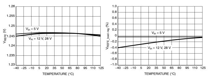
Figure 15. External Reference Voltage vs. Input Voltage and Temperature
