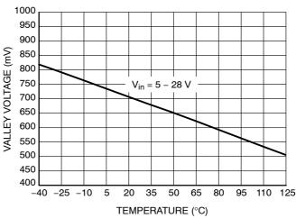
Figure 14. Valley Voltage vs. Input Voltage and Temperature
