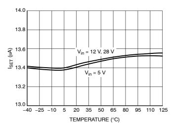
Figure 17. Current Limit Set Current vs. Temperature
