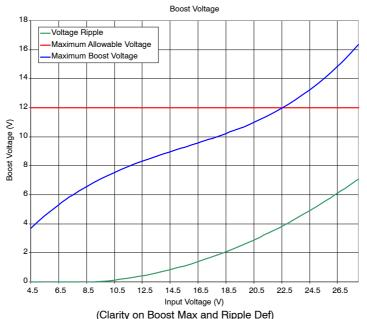
Figure 32. Boost Voltage at 80% Duty Cycle
