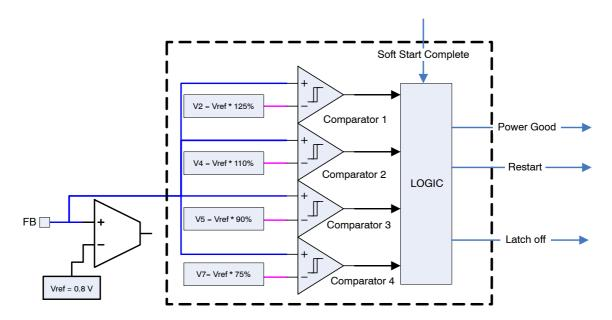
Figure 23. OOV, OUV, and Power Good Circuit Diagram
