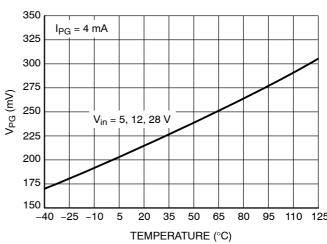
Figure 10. Power Good Output Low Voltage vs. Input Voltage and Temperature
