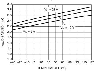
Figure 5. Supply Current vs. Input Voltage and Temperature
