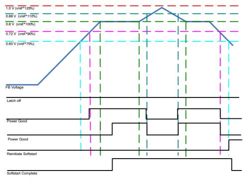
Figure 26. Powerup Sequence and Undervoltage Soft-Start
