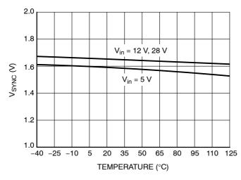
Figure 13. SYNC Threshold vs. Input Voltage and Temperature
