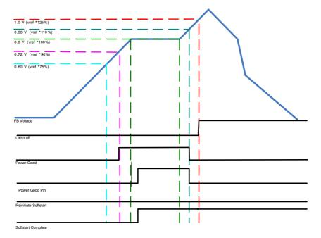
Figure 25. Powerup Sequence and Overvoltage Latch
