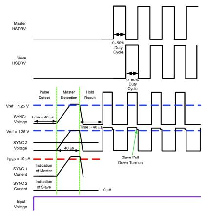
Figure 21. Master Slave Typical Waveforms
