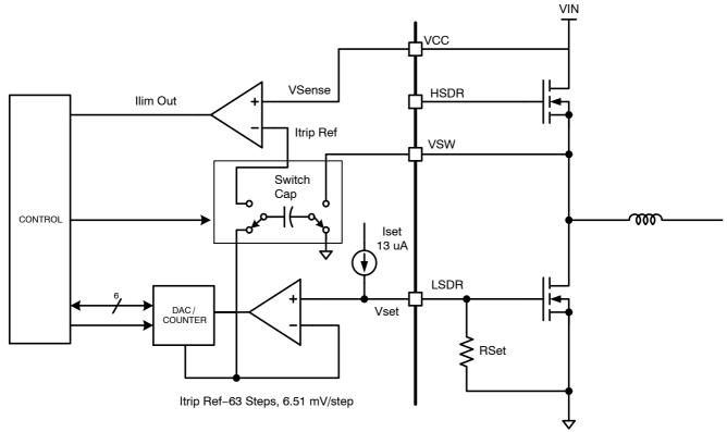
Figure 27. I<sub>set</sub> / I<sub>Limit</sub> Block Diagram
