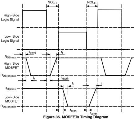
Another consideration during MOSFET selection is their delay times. Turn-on and turn-off times must be short enough to prevent cross conduction. If not, there will be conduction from the input through both MOSFETs to ground. Therefore, the following conditions must be met.
