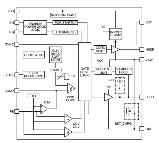
Figure 2. NCP3012 Block Diagram
