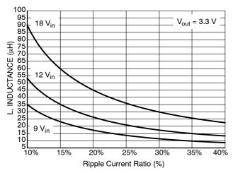
Figure 33. Ripple Current Ratio vs. Inductance
