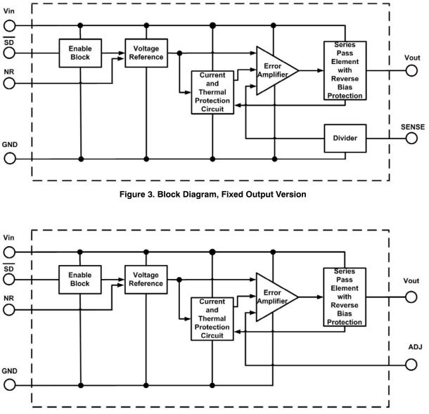
Figure 4. Block Diagram, Adjustable Output Version
