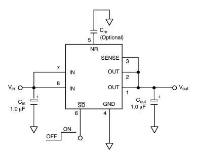
Figure 1. Typical Fixed Version Application Schematic (Micro8 Package)
