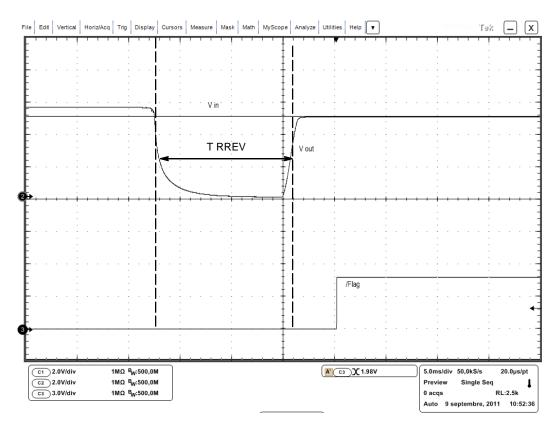
Figure 16. Reverse Voltage Removal
