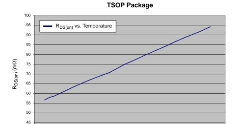
Figure 20.  $R_{DS(on)}$  vs Temperature, TSOP Package
