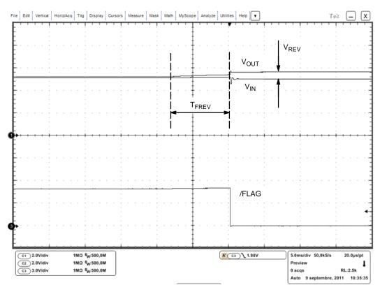
Figure 15. Reverse Voltage Detection
