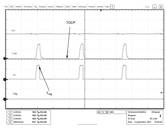
Figure 11. Timer Regulation Sequence During 2  $\Omega$  Overload
