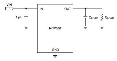
Figure 3. Test Configuration
