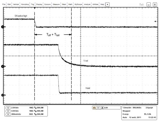
Figure 7. Toff Delay and Tfall
