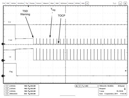
Figure 9. 2  $\Omega$  Short on Output. Complete Regulation Sequence
