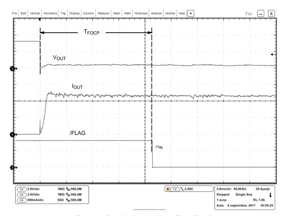
Figure 14. From No Load to Direct Short Circuit
