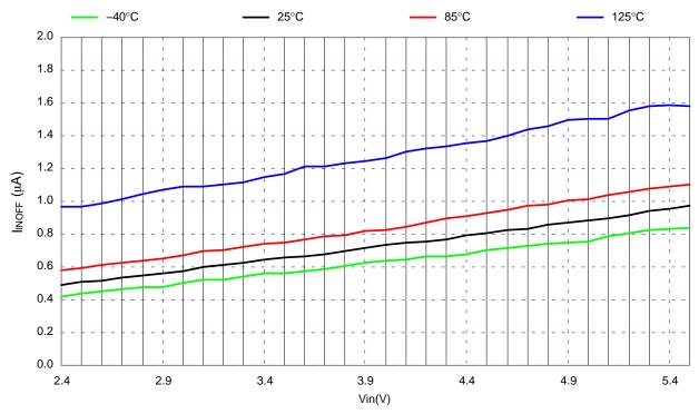
Figure 18. Standby Current vs Vin
