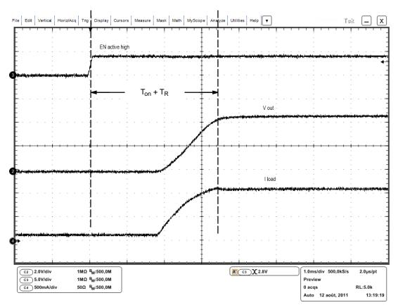
Figure 6.  $T_{on}$  Delay and  $T_{rise}$  Time
