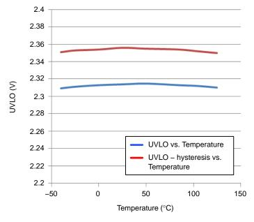
Figure 17. Undervoltage Threshold (Falling) and Hysteresis
