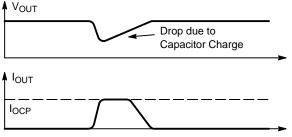
Figure 22. Heavy capacitive load
