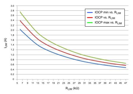
Figure 26. Current Threshold vs. Rlim Resistor
