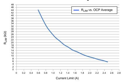
Figure 25.  $R_{\text{LIM}}$  Curve vs. Current Limit
