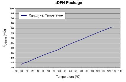
Figure 21.  $R_{DS(on)}$  vs Temperature,  $\mu DFN$  Package
