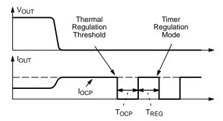
Figure 24. Short circuit
