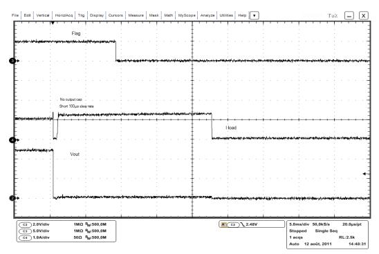
Figure 12. Direct Short on OUT Pin
