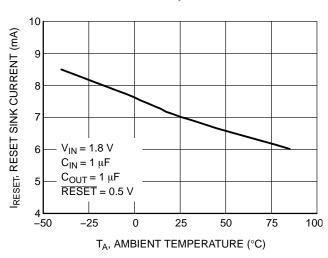
Figure 12. RESET Pin N-Channel Sink Current vs. Temperature
