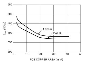
Figure 22.  $\theta_{\text{JA}}$  vs. Copper Area
