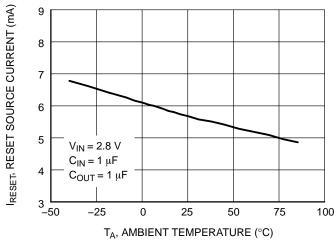
Figure 13. RESET Pin P-Channel Source Current vs. Temperature
