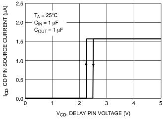
Figure 19. Delay Pin Source Current vs. Voltage
