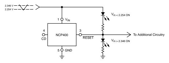
Figure 26. Input Voltage Indicator
