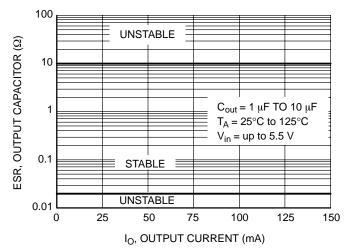
Figure 25. Output Capacitor versus Output Current
