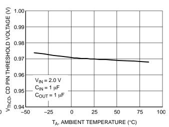
Figure 14. CD Delay Pin Threshold Voltage vs. Temperature
