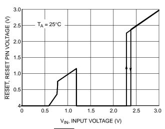
Figure 18. RESET Pin Voltage vs. Input Voltage
