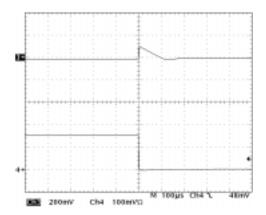
$I_{OUT}$  = 150 mA to 1 mA,V $_{IN}$  = 3.3 V,  $C_{IN}$  = 1  $\mu F$  Upper Trace: Output Voltage 200 mV/div Lower Trace: Output Loading Current 100 mA/div
