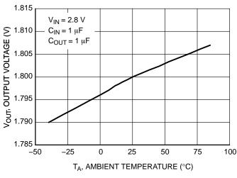
Figure 7. Output Voltage vs. Temperature
