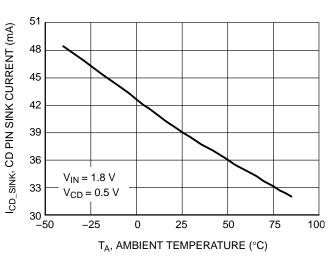
Figure 16. CD Pin Sink Current vs. Temperature
