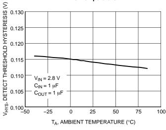
Figure 11. Dectector Threshold Hysteresis Voltage vs. Temperature
