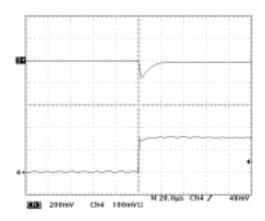
$I_{OUT}$  = 1 mA to 150 mA,V $_{IN}$  = 3.3 V,C $_{IN}$  = 1  $\mu$ F Upper Trace: Output Voltage 200 mV/div Lower Trace: Output Loading Current 100 mA/div
