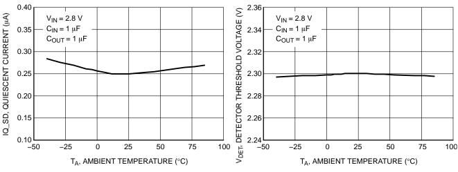
Figure 9. Quiescent Current (Shutdown) vs. Temperature
