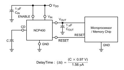
Figure 27. Microprocessor Reset Circuit
