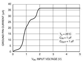
Figure 17. Ground Pin Current vs. Input Voltage
