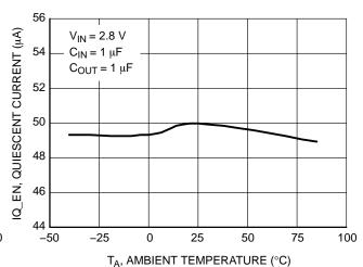
Figure 8. Quiescent Current (Enable) vs. Temperature
