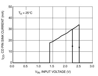
Figure 20. CD Pin Sink Current vs. Input Voltage
