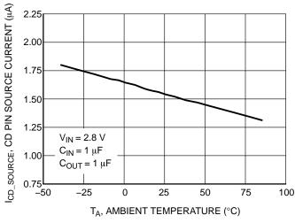
Figure 15. CD Pin Source Current vs. Temperature
