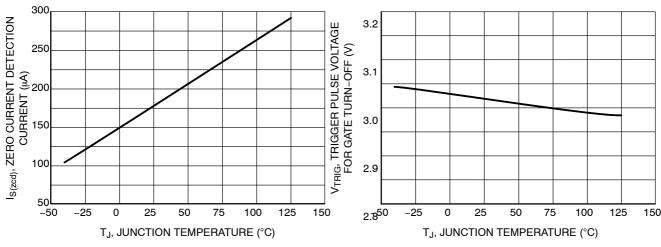
Figure 13. Zero Current Detect I<sub>source</sub> vs. **Junction Temperature**
