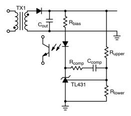
Figure 29. Typical Secondary Side Regulator
