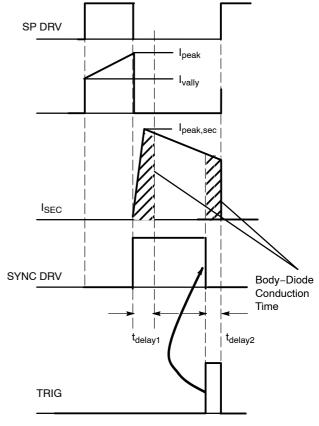
Figure 32. Continuous Conduction Mode Waveforms
