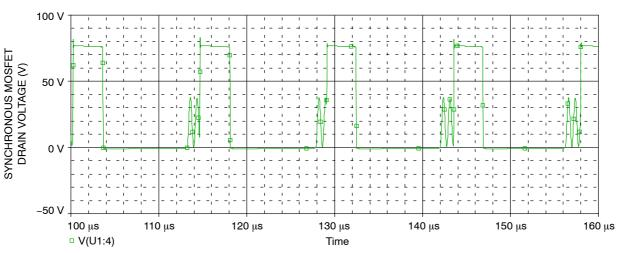
Figure 28. Discontinuous Conduction Mode Drain Waveform
