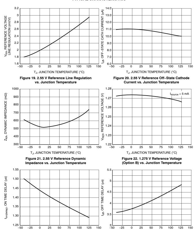
$\label{eq:total_total} T_J, \mbox{ JUNCTION TEMPERATURE (°C)}$  Figure 23.  $t_{on}$  Delay vs. Junction Temperature
