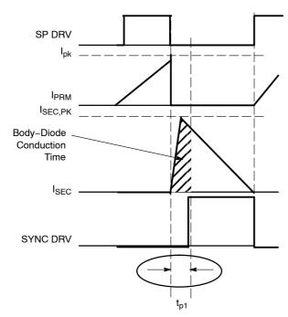
Figure 31. Discontinuous Conduction Mode Waveforms
