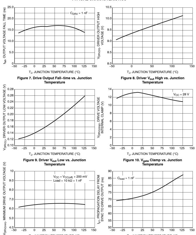
TJ, JUNCTION TEMPERATURE (°C) Figure 11. V<sub>OUT(min)</sub> vs. Junction Temperature
