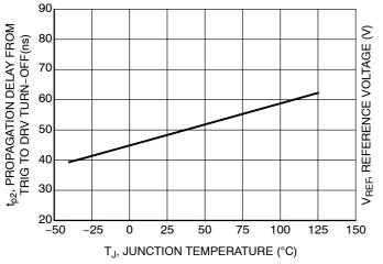
Figure 15.  $t_{\rm p2}$  Propagation Delay TRIG in to DRIVE Off, NO Load vs. Junction Temperature
