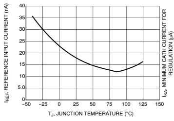
Figure 17. 2.55 V Reference Input Current vs. **Junction Temperature**
