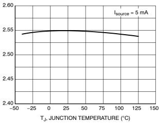
Figure 16. 2.55 V Reference (Option A) Voltage vs. Junction Temperature
